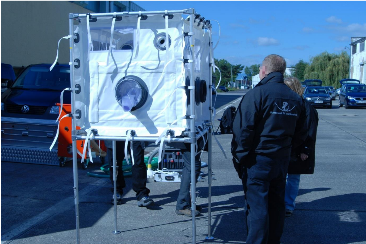
FIG. 3. Glove box for the examination of contaminated evidence from the crime scene. The evidence gets introduced through the round opening visible at the front of the picture. A panel providing multiple connections for electronic equipment can be attached to the other side of the glove box in case a laptop or mobile phone need to be examined and data extracted.
