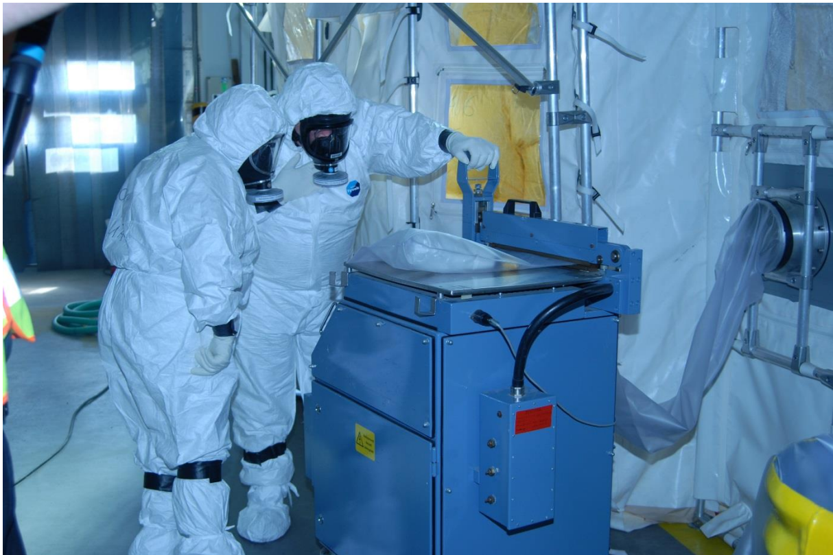
FIG. 2. Airlock with a plastic sleeve in which the contaminated evidence from the crime scene can be heat sealed by means of the heat sealing machine. The heat sealing machine is set up on wheels so it can be transferred to the glove box when necessary.
