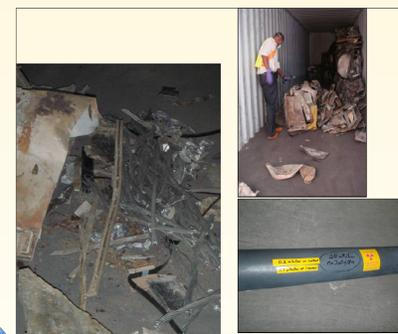
Source Recovery and Inspection for a Gamma Alarm. Static Eliminator, a Ra-226 lined H-Strip of Metal
