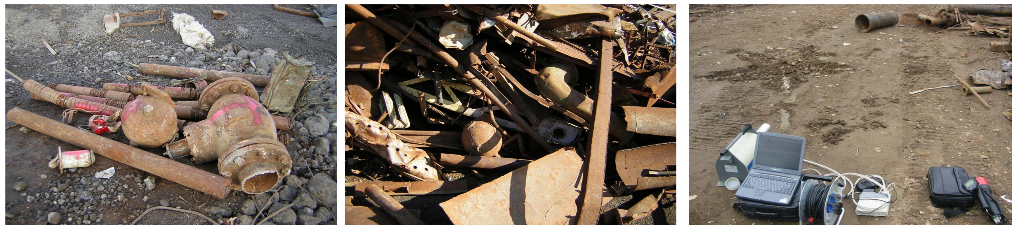
Radioactive objects located in the scrap metal load
