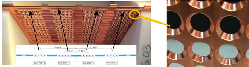
FIG. 6. Production of Plasma Grid segment (showing the angled configuration) and the apertures
