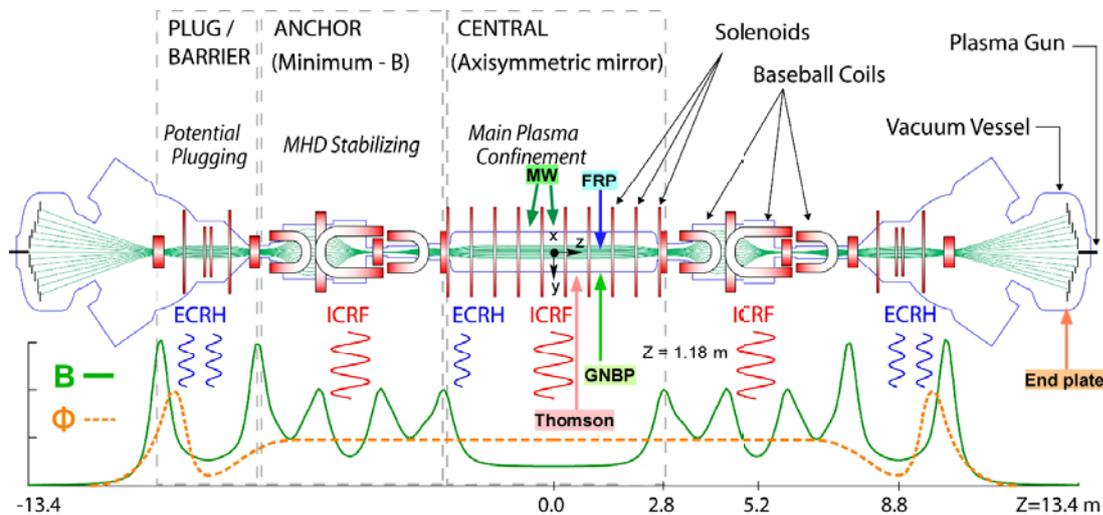
FIG. 1. Schematic view of GAMMA 10/PDX.
