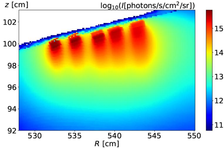
FIG. 5. A synthetic diagnostic measurement at arbitrary camera location for the Helium 667.8 nm line intensity from five simulated He beams in the vicinity of an upper Wendelstein 7-X island divertor.
