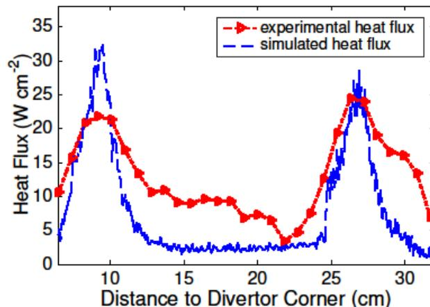
FIG. 3. Experimental (red) and simulated (dashed blue) heat flux on the lower outer divertor. The position of the infrared camera is indicated by the vertical dashed orange line in Fig. 2.
