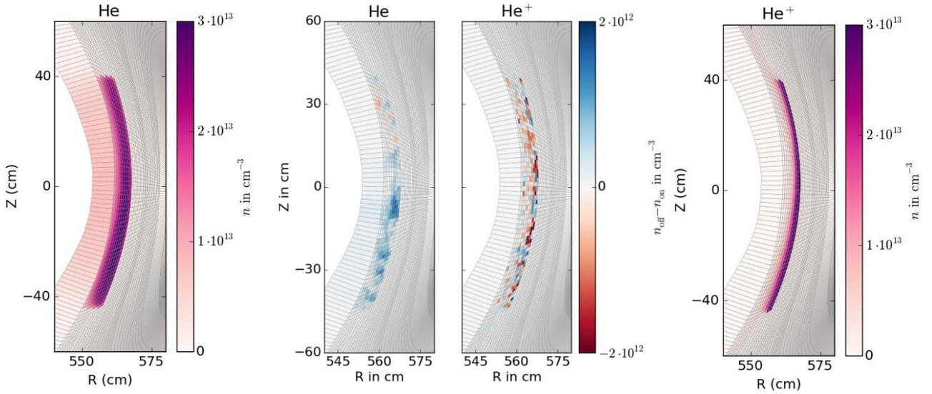
FIG. 7. Poloidal profiles of atomic (left) and minority ion density (right) obtained by classic kinetic ion treatment. Center: absolute difference (up to 10%) between atomic and ionic densities at the limiter (fixed toroidal angle).
