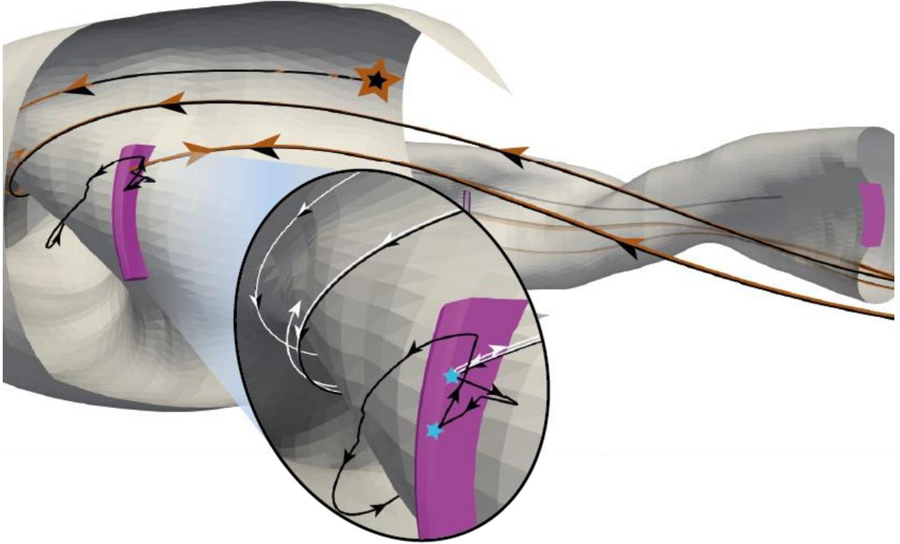
FIG. 6. Single  $\text{He}^+$  trajectory for classic EIRENE ion transport (brown, white in inset) compared to enhanced transport (black) with the starting location indicated by the star. In the latter case, the test ion reflected at the limiter (in purple) turns due to the mirror force and follows its pre-impact direction. In classic ion transport, the test ion reflect off the limiter into almost the same trajectory it came from (arrows highlight the direction of flow).
