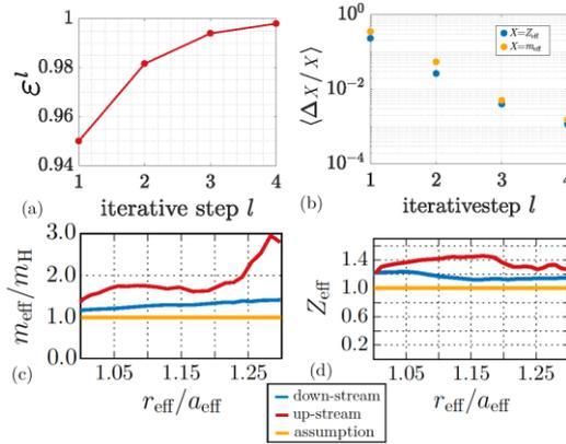
FIG. 4. Iterative process adjusting the separatrix density to find a converged effective mass and charge state. Radial profile of  $Z_{\text{eff}}$  and  $m_{\text{eff}}$  at the down- and up-stream location, showing significant deviations outside the last closed flux surface. The upper plots show the convergence behavior of the abovementioned iterative scheme.
