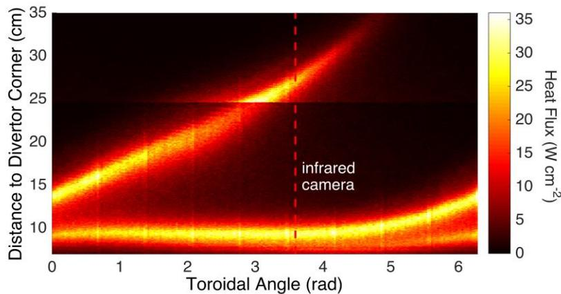
FIG. 2. Simulated heat flux footprint on the lower outer divertor targets.
