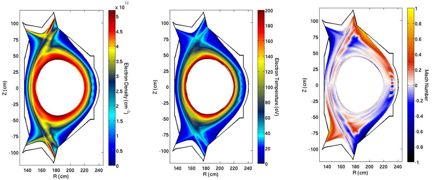
FIG. 1. The poloidal cross-sections of the electron density, electron temperature and Mach number simulated by the EMC3-EIRENE code at the same toroidal position with the LHW antenna for a perturbed (by RMPs) plasma.
