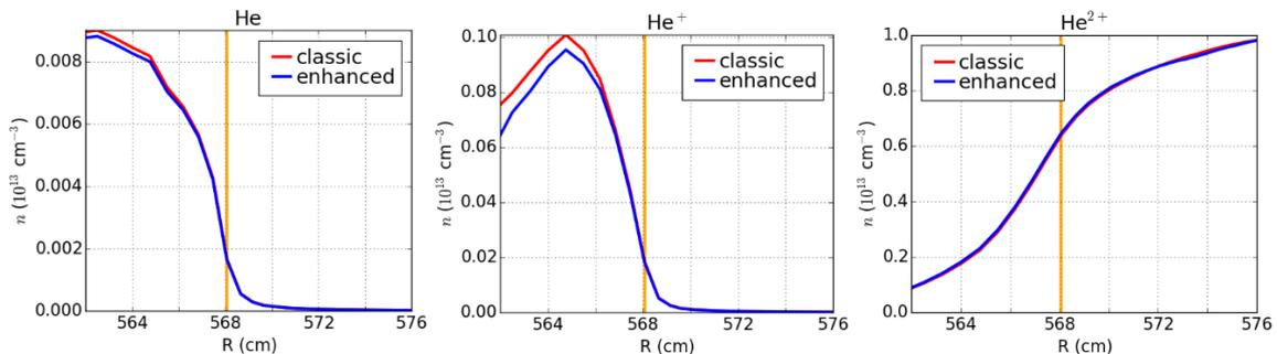
FIG. 8. Toroidally and poloidally averaged radial profiles of the different helium densities, obtained using classic and enhanced transport in EIRENE for He<sup>+</sup>.
