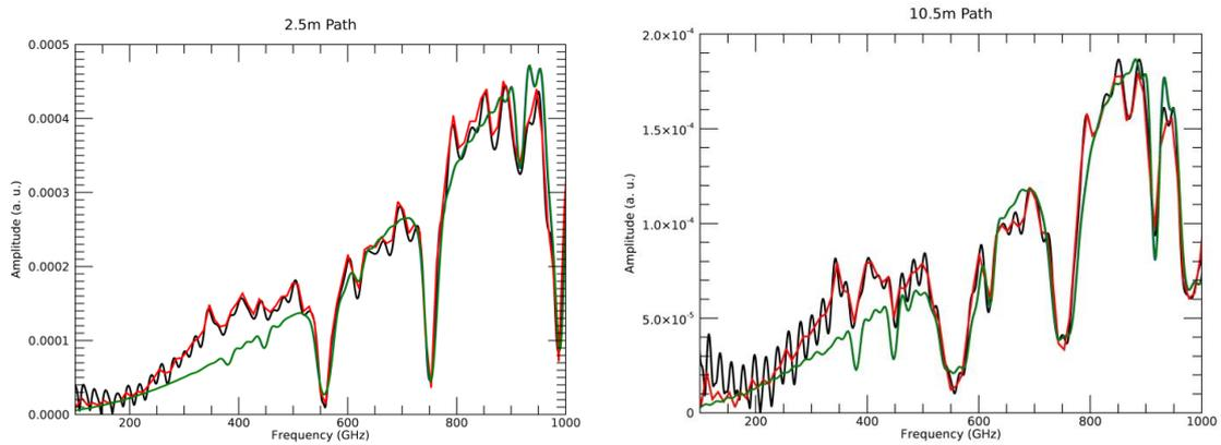
FIG.7. Comparison of measured (red) and simulated (green) spectra for total paths of 2.5 m (left) and 10.5 m (right).
