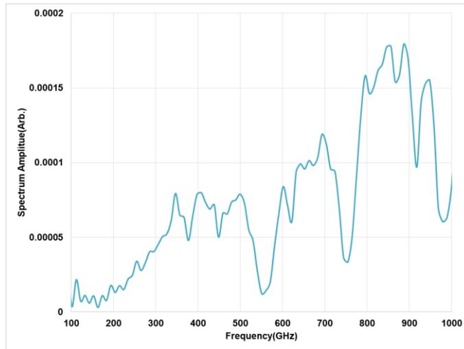
FIG.3. the spectrum profile of the liquid nitrogen temperature black body source
