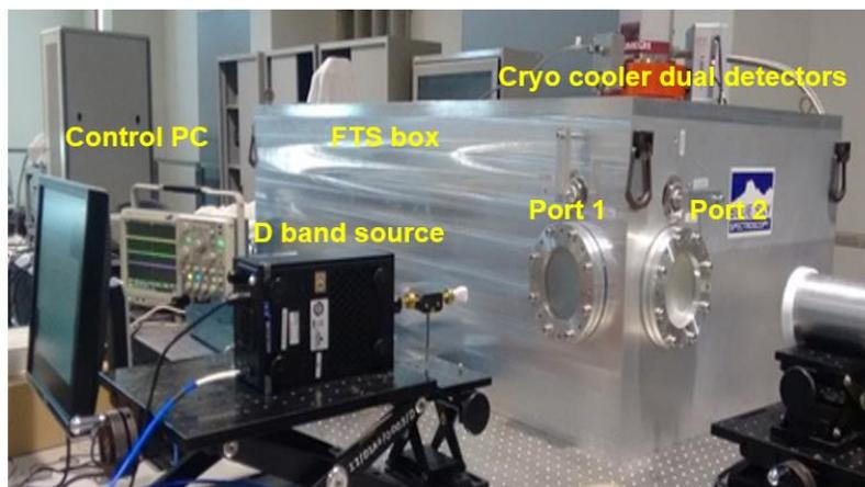
FIG. 2. Photograph of the ECE spectrometer showing sources and inputs
