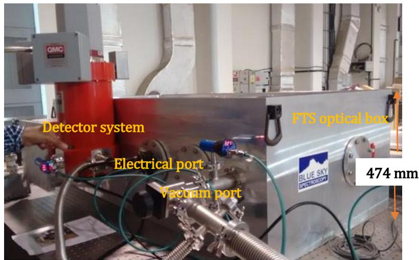
FIG.1. Photograph of the ECE spectrometer identifying key components
