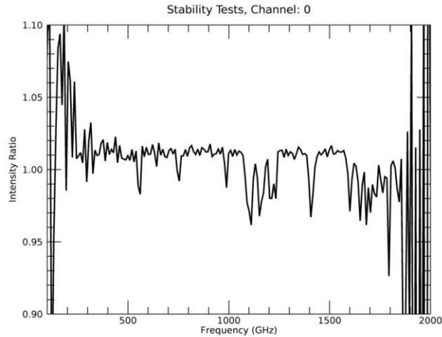
FIG.5. the stability of the FTS expressed as the ratio of spectra taken 19 hours apart. Large variations correlate with the position of water vapour lines indicating that environmental effects dominate the current stability measurements
