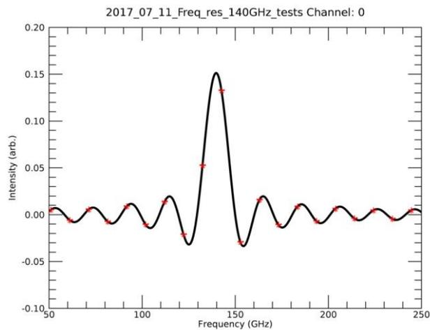
FIG.4. Phase corrected (red symbols) and zero-padded spectrum (black) of the 140 GHz line source showing classical sinc instrumental line shape.
