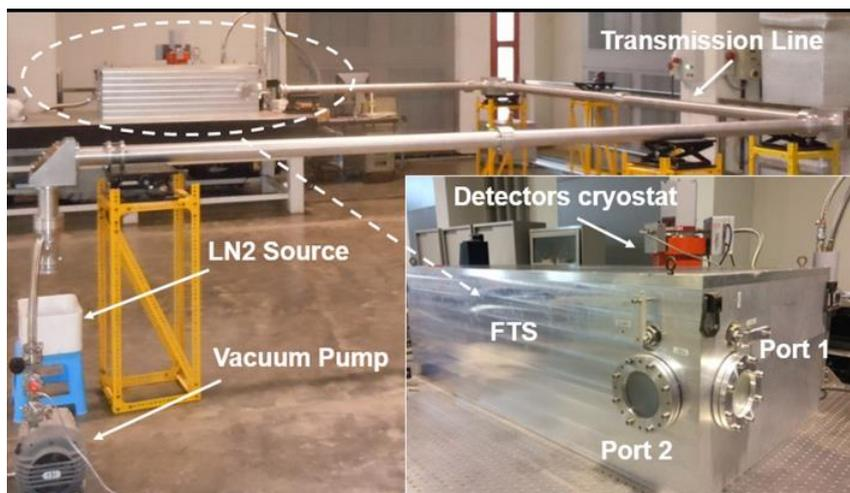
FIG.6. Experimental configuration for the transmission line attenuation measurement
