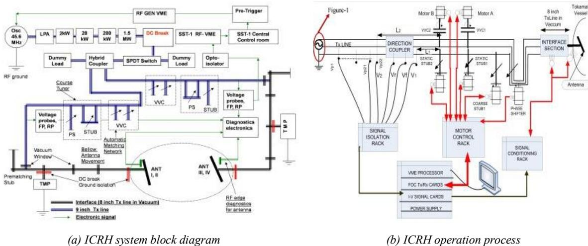
(a) ICRH system block diagram
