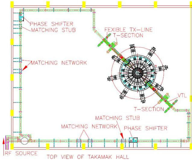
FIG. 1. ICRF Tx-line layout in SST-1 tokamak
