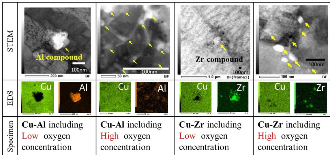
Figure2. STEM image and EDS chemical mapping for Cu and Al, Zr for the alloy with MA for 32~40 hrs and HIP.
