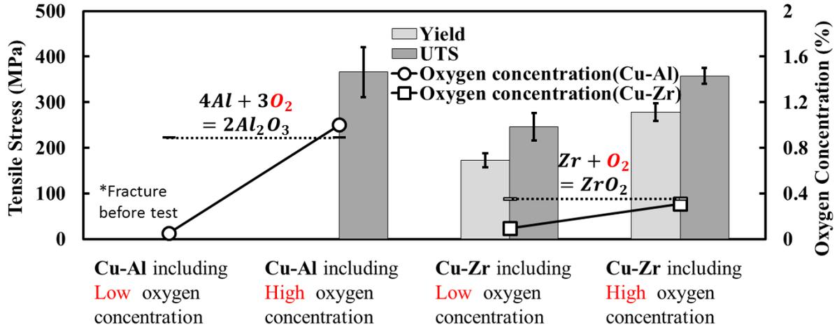
Figure1. Effects of oxygen concentration on mechanical properties and microstructure for Cu-Al and Cu-Zr.
