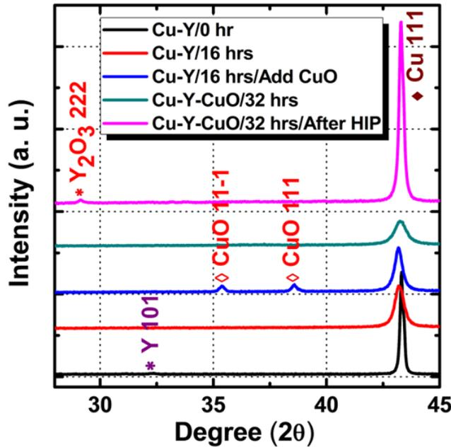
Figure 3. XRD spectra showing the evolution of crystal information of the Cu-Y and Cu-Y-CuO powders during the MA-HIP process.
