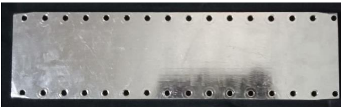
FIG. 10. Fabricated Covering plate of the step phase shifter.
