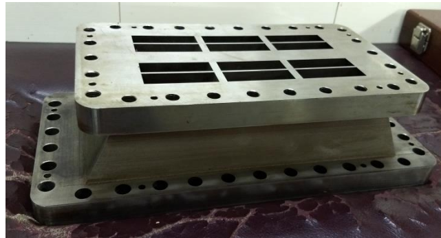
FIG. 4. Tapered Divider after EDM Wire Cutting process.
