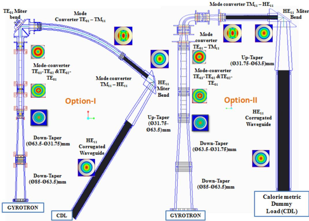
Fig.1. Schematic of design approaches of proposed transmission line system
