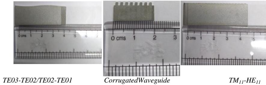
Fig.2. Pre-fabrication samples of mode converters and corrugated waveguide
