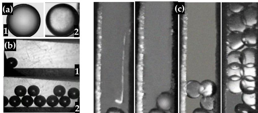
FIG. 3. Results of the FST-LM operation with a rate of 0.1 Hz at 5.0 K. In (a) FST-layering result: 1 – 40- $\mu\text{m}$ -thick  $D_2$  layer with 20% Ne additives in free-standing CH shell of 1.23-mm diameter (20% Ne in order to modeling the D–T fuel), 2 – 44- $\mu\text{m}$ -thick  $H_2$  layer with 5% HD additives in free-standing CH shell of 1.2-mm diameter; in (b) horizontal TC: 1 – 1 target (0 s), 2 – 10 targets (100 s); in (c) vertical TC: 12 targets (100 s).
