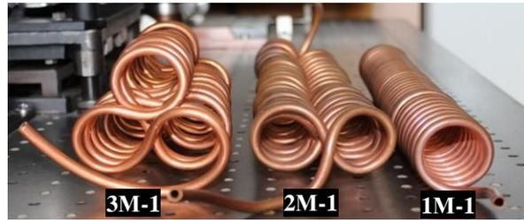
FIG. 4. Different geometry of the LC mockups used in the FST layering module.
