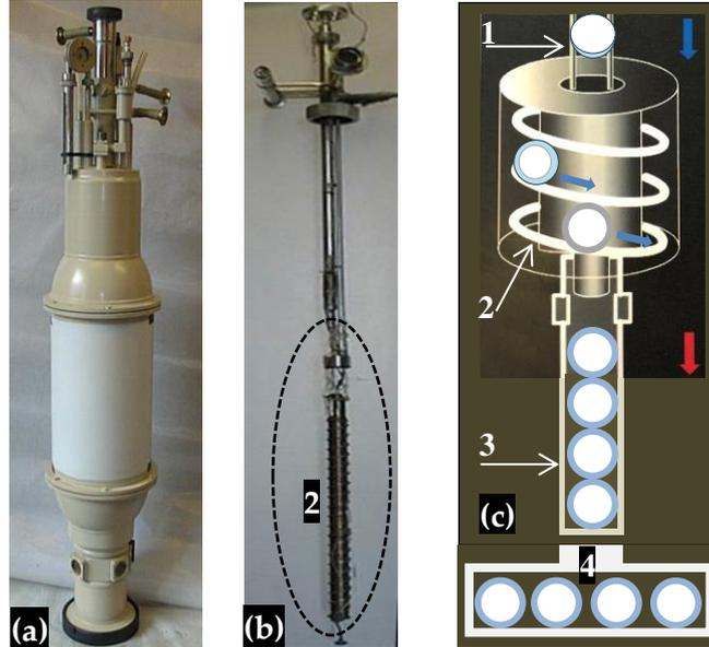
FIG. 2. FST-LM: (a) overview, (b) single spiral LC in assembly, (c) schematic of the repeatable operation of the FST-LM: 1 – gravitation loading of the target with liquid fuel from the SC to the LC, 2 – LC, 3 – vertical target collector, 4 – horizontal target collector.
