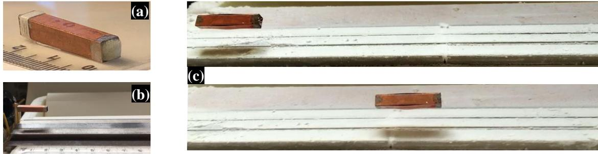
FIG. 6. HTSC-sabot friction-free acceleration by the driving electromagnetic pulse generated by the field coil: (a) HTSC-sabot overview; (b) HTSC-sabot before acceleration; (c) in-time development of the acceleration process.
