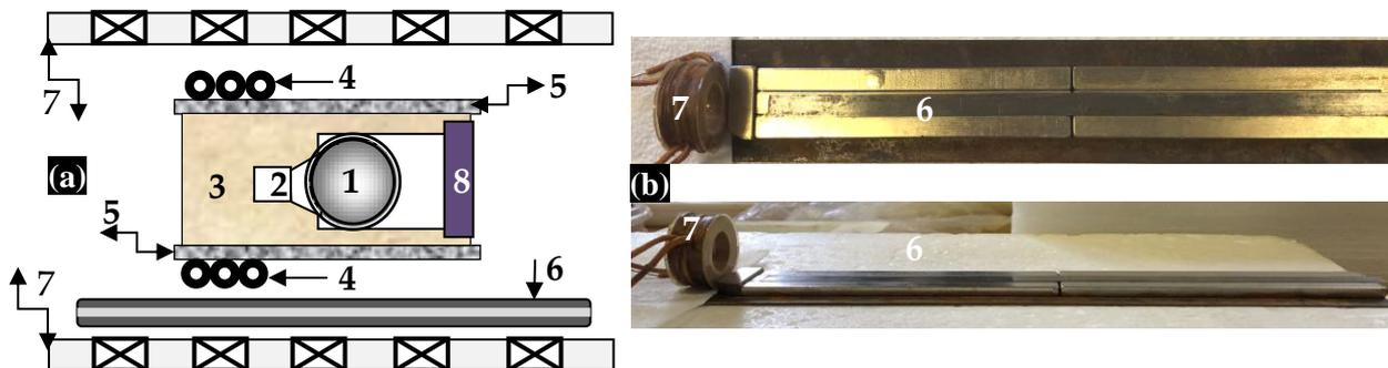
FIG. 5. Schematic of «EM-AC + PMG» accelerator. In (a): 1 – target, 2 – conical support for the target nest, 3 – sabot matrix (polymer), 4 – HTSC-coils (driving body based on superconducting  $MgB_2$ -cables), 5 – HTSC-plates for providing a stable levitation along the magnetic track, 6 – magnetic track, 7 – field coils, 8 – protective cover; in (b): experimental setup (top and side view).
