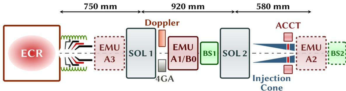
FIG. 1. LIPAC ion source and LEBT set-up. Different positions of the emittance meter are shown for the different phases of the beam commissioning.
