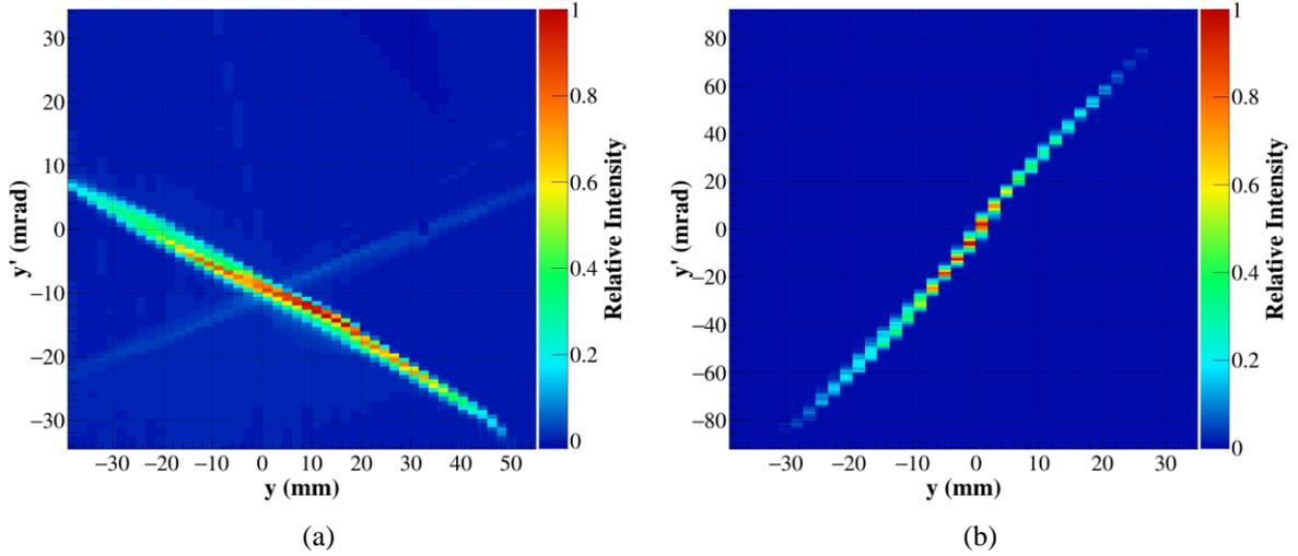
FIG. 2. Beam distribution measurement in the  $(yy')$  phase space of a 140 mA  $D^+$  beam at 100 keV at two positions of the LIPAc LEBT (a): A1 phase measurement – (b): A2 phase measurement
