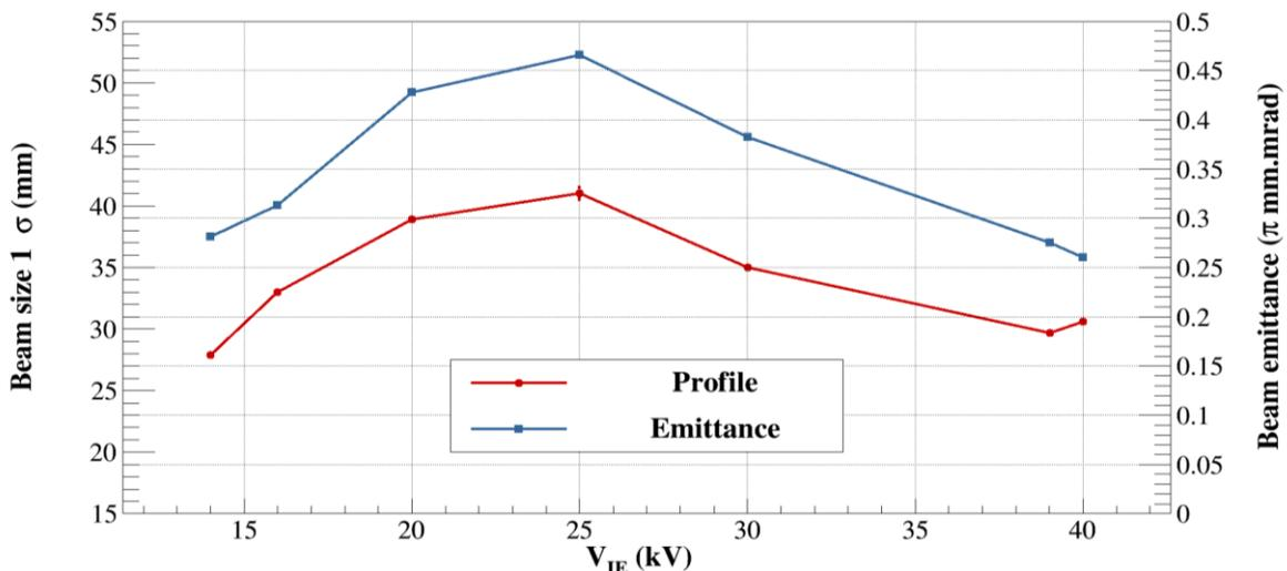
FIG. 3. Beam size ( $1\sigma$ ) and emittance versus intermediate electrode voltage.
