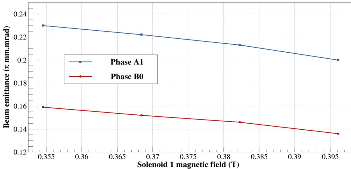
FIG. 4. Beam emittance versus magnetic field applied by solenoid 1. Comparison of phase A1 and B0 measurements.
