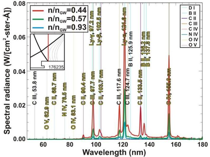
FIG. 4. Spectral radiance with 290 g/mm grating viewing the OSP at various  $n/n_{GW}$ . Resonance lines are labeled in bold with yellow text.
