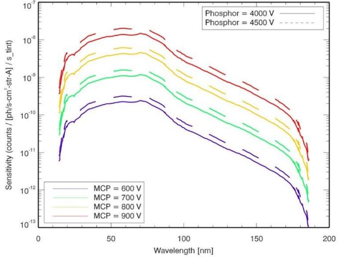
FIG. 3. Spectrometer sensitivity vs. wavelength for DivSPRED with 290 gr/mm grating and increasing MCP and phosphor high voltage.
