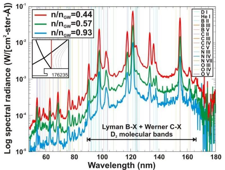
FIG. 7. Same spectral radiance with 290 g/mm grating viewing the OSP at increasing  $n/n_{\text{GW}}$  as shown in FIG. 3. A log Y-axis reveals many additional emission lines, and a region where Lyman-Werner  $D_2$  bands may account for missing radiation compared to modeling.
