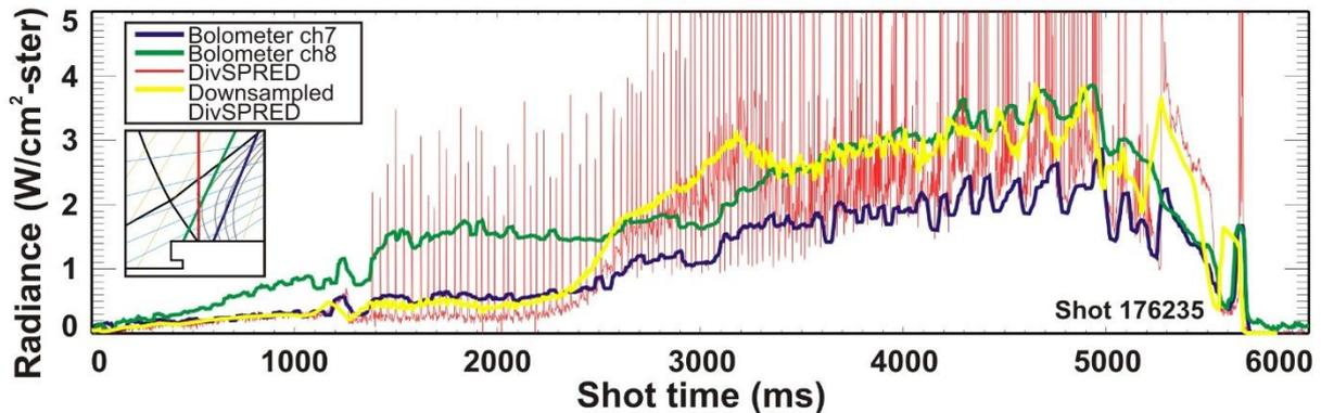
FIG. 5. Integrated radiance through full DivSPRED spectrum for a density ramp discharge. DivSPRED data is taken at 544 Hz (red), then down-sampled to 25 Hz (yellow) to compare to neighboring bolometer channels (green and purple).
