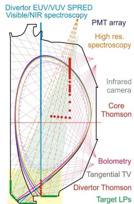
FIG. 1. Diagnostic suite for the DIII-D divertor used for radiation studies.
