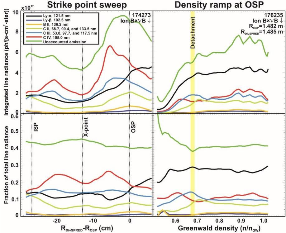
FIG. 6. Integrated line radiance for major emission lines (top) and fractional emission of the total (bottom) for both a strike point sweep at constant density (left) and a density ramp with a steady strike point (right) as measured by DivSPRED.
