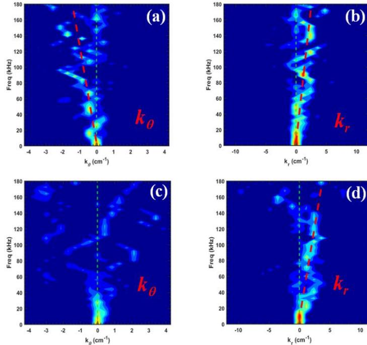
FIG. 3. Wavenumber-frequency structure for low- $q$  large current discharge (a) in electron diamagnetic direction, (b) in outward direction and for low current tokamak discharges (c) with center concentration, (d) in outward direction
