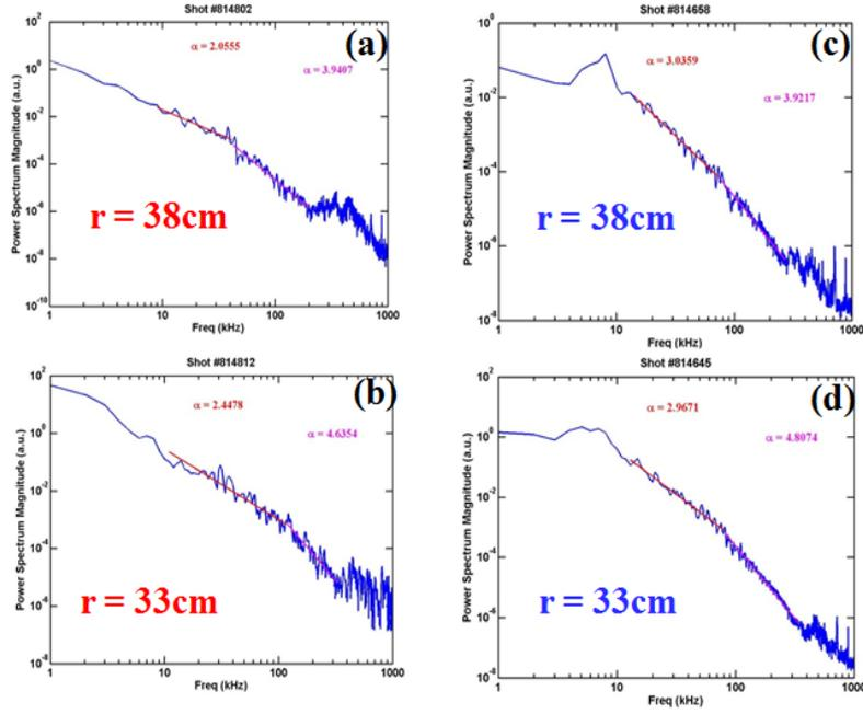
FIG. 2. Energy spectra of floating potential in low  $q$  high current discharge (a) at radial position  $r=38$ , (b) at radial position  $r=33$ , and in low current tokamak discharge (c) at radial position  $r=38$ , (d) at radial position  $r=33$
