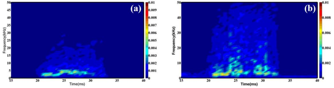
FIG. 6. Frequency spectrum of (a) center chord averaged electron density, (b) electron density fluctuation by forward scattering in low current tokamak discharge
