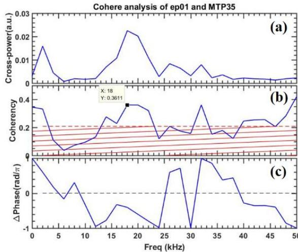
FIG. 5. In low current tokamak discharge, (a) corss power, (b) coherency and (c) phase difference between floating potential fluctuation and edge Bp fluctuation,
