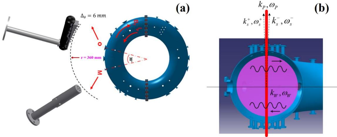
FIG. 1. (a) Diagram of edge probes arrangement on KTX vacuum vessel windows, (b) Diagram of the forward scattering signal collection on KTX
