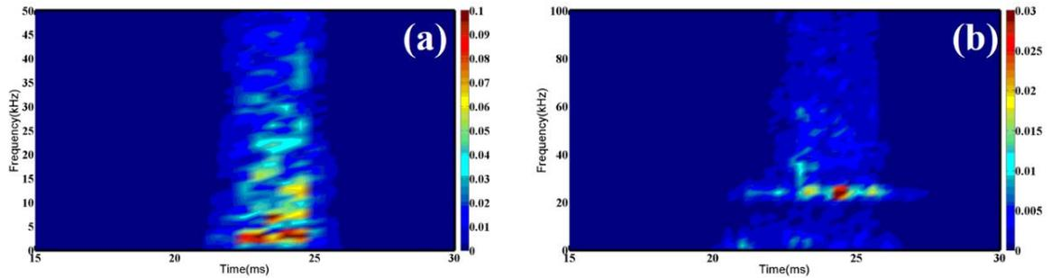
FIG. 7. Frequency spectrum of (a) electron density fluctuation by forward scattering, (b) Bp edge mirnov probe in reversed field pinch discharge
