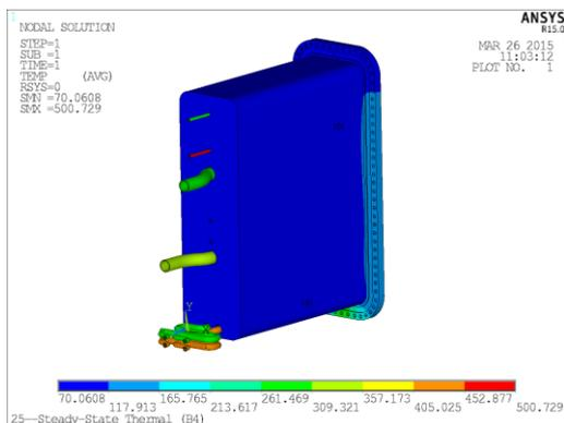
FIG. 15 Temperature distribution on TBM shield
