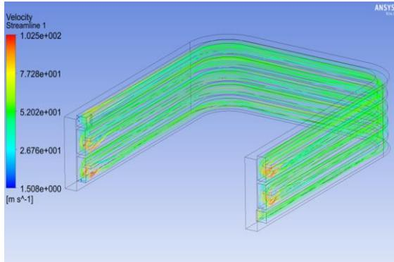
FIG. 5 Velocity streamlines in the FW cooling channel
