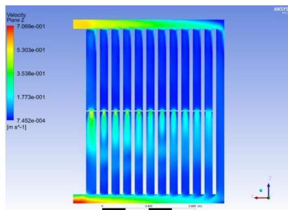
FIG. 12 Velocity plot in the mid-plane
