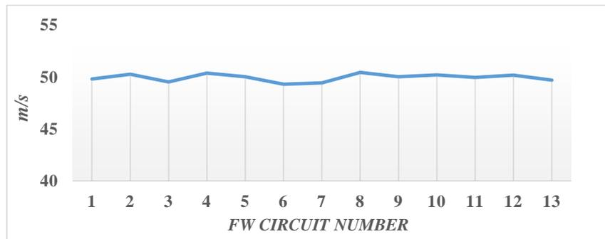
FIG. 4 Flow velocity in parallel FW circuits
