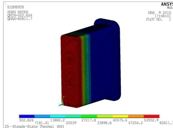
FIG. 14 Heat generation plot in TBM shield
