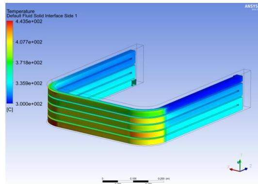
FIG. 8 Channel wall temperature of FW
