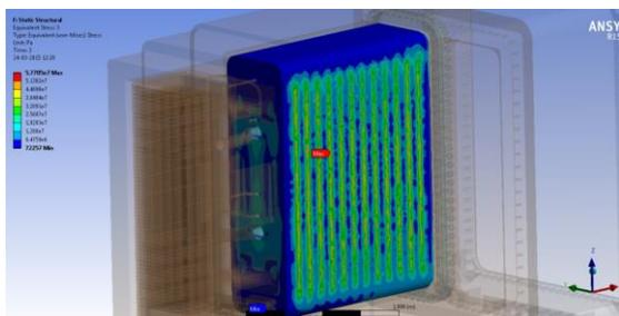
FIG.19 von mises stress plot in shield due to primary load
