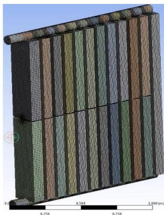
FIG. 11 Water flow model in TBM shield
