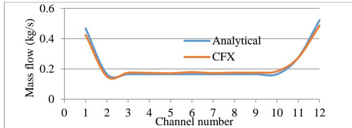
FIG. 13 Comparison between analytical and CFX calculated mass flow
