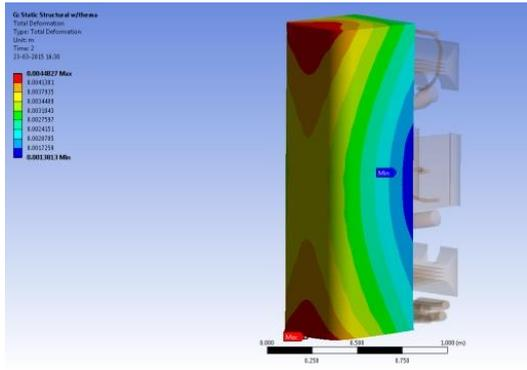
FIG. 17 Displacement plot in TBM
