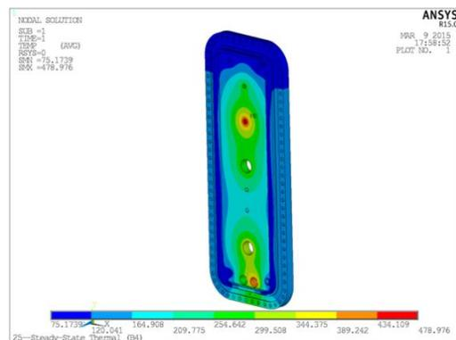
FIG. 16 Temperature distribution of TBM set flange
