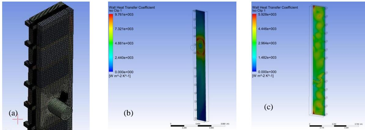
FIG. 10(a) Model for helium manifolds, (b) HTC plot for inlet manifold, (c) HTC plot for outlet manifold
