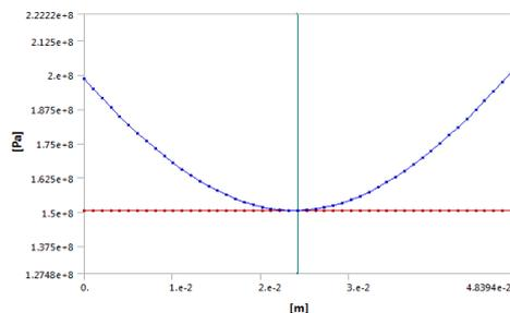
FIG.20 Stress linearization for primary and secondary loads
