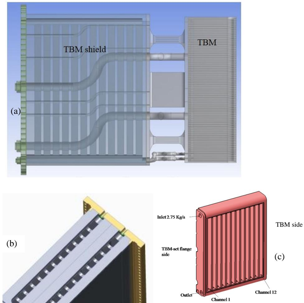
FIG. 1 a) LLCB TBM set b) Inlet manifolds in shield and c) water flow arrangement in one half of TBM shield
