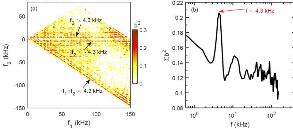
FIG. 4. (a) Contour-plot of squared auto-bicoherence of the envelope of density fluctuations  $b^2(f_1, f_2)$ , and (b) the summed bicoherence for each frequency  $f$ .
