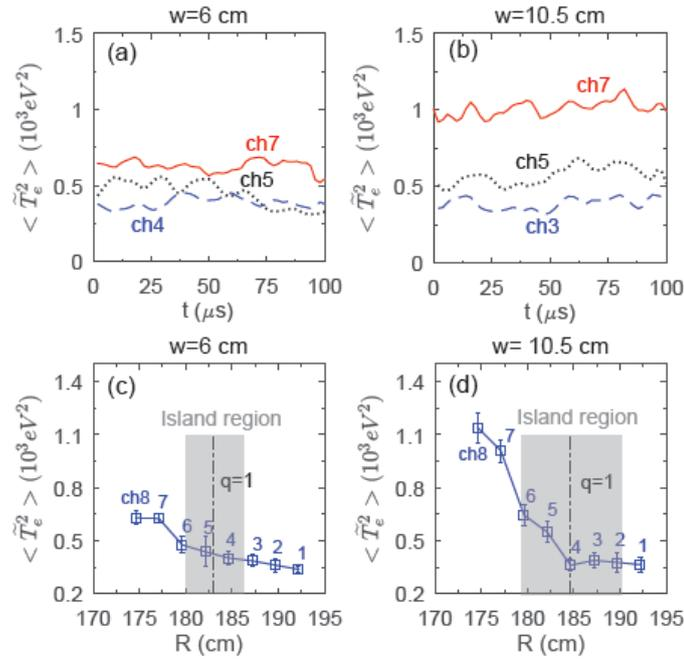
FIG. 6. Temporal evolutions of the  $T_e$  fluctuation power,  $\langle \tilde{T}_e^2 \rangle$ , measured on several ECEI channels at  $Z=3.46$  cm across the O-point phase for two different island widths (a)  $w=6$  cm and (b)  $w=10.5$  cm. (c) and (d) show the radial profiles of  $\langle \tilde{T}_e^2 \rangle$  measured by eight channels in Fig. 5(a) for  $w=6$  cm and  $w=10.5$  cm, respectively.
