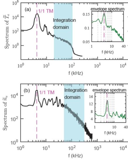
FIG. 3. Power spectrum of (a)  $\tilde{T}_e$  and (b)  $\tilde{n}_e$ . The inset in (a) and (b) shows the amplitude spectrum of the corresponding envelope signal,  $\phi_{\tilde{T}_e}(t)$  in the frequency range  $\Delta f=20-100$  kHz (shaded in (a)) and  $\phi_{\tilde{n}_e}(t)$  in  $\Delta f=50-300$  kHz (shaded in (b)), respectively.
