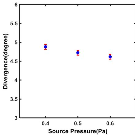
Fig. 5a. The effect of source filling pressure on the beam divergence.
