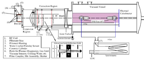
Fig. 1a. ROBIN test stand (source and vacuum vessel) with the spectrometer.
