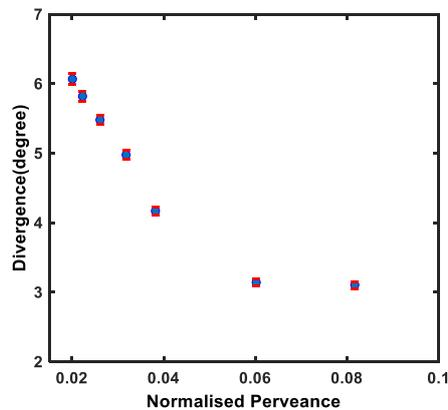
Fig.3. The normalized perveance condition of the beam at 12 kV acceleration voltage, 40 kW RF power and 0.6 Pa source pressure
