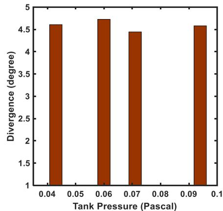
Fig. 5b. The effect of tank pressure on the beam divergence.
