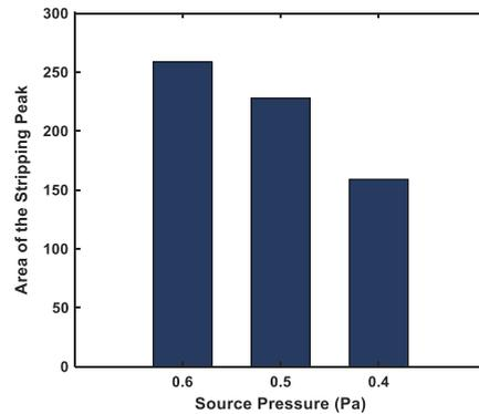
Fig. 8b. The area under curve of the stripping peak at 17 kV total grid voltage at 40 kW RF power.
