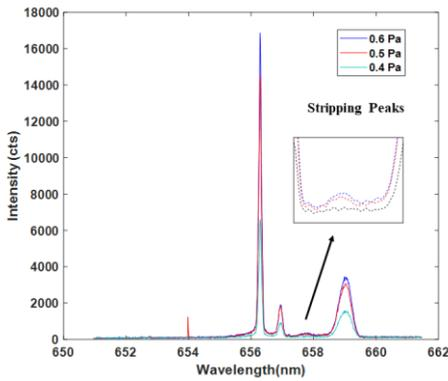
Fig. 8a. The spectrum for shots at three different pressures (0.6, 0.5, 0.4 Pa) showing the stripping peaks
