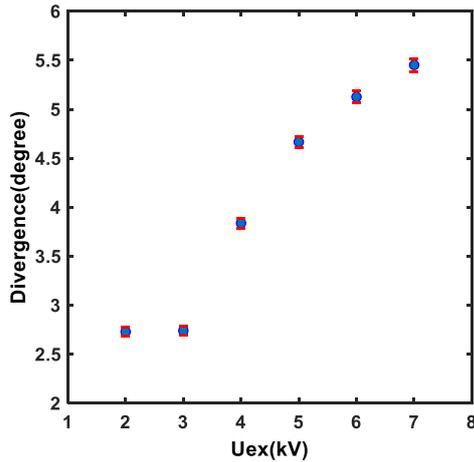
Fig. 6a. The variation of the divergence with the voltage applied across the extraction grid ( $U_{ex}$ ) at  $U_{acc} = 12$  kV, RF Power = 40 kW and source pressure = 0.6 Pa.
