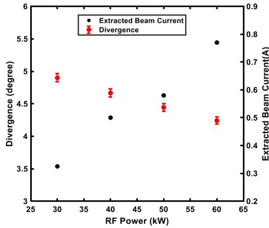
Fig. 4. The divergence and the extracted beam current variation with the RF at 17 kV total applied voltage in the grid.
