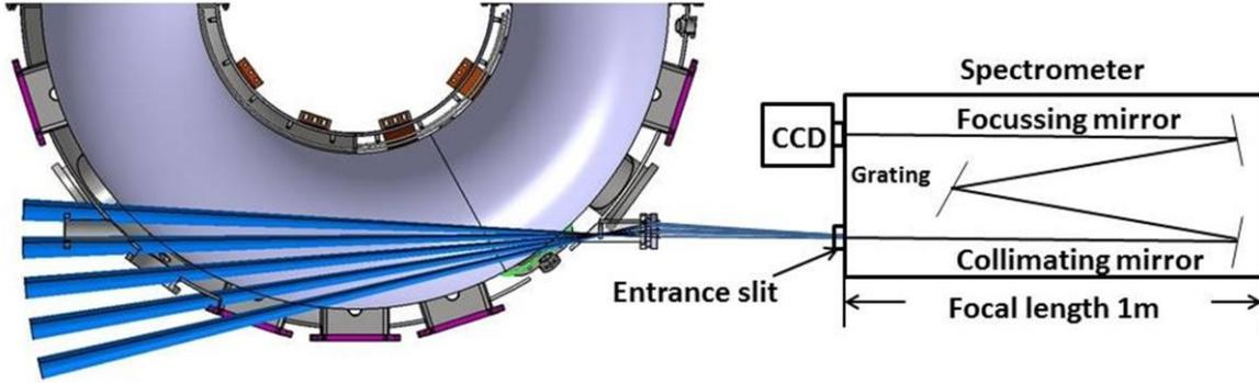
FIG. 1. Experimental set up showing arrangement of line of sights for toroidal rotation measurement .
