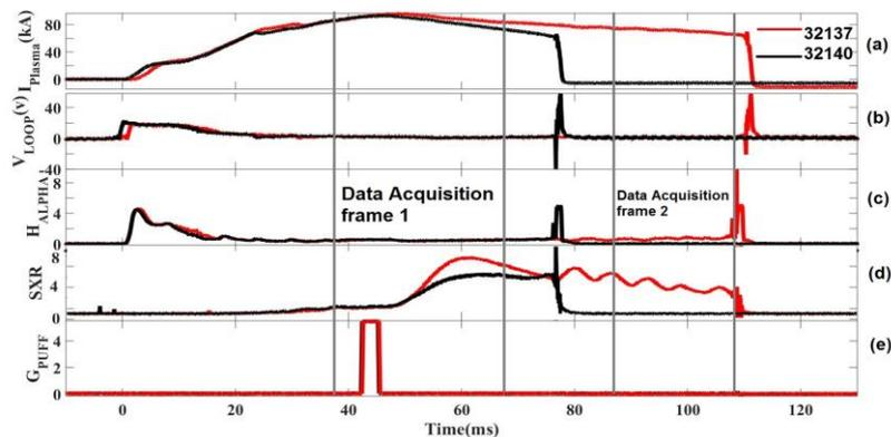
FIG. 3. Typical ADITYA-U discharge of shot #32140 along with CCD exposure duration.(a) Plasma current, (b) loop voltage (V), (c)  $H_\alpha$  emission (d) soft X-ray emission(SXR) and (e) Gas puff pulse.
