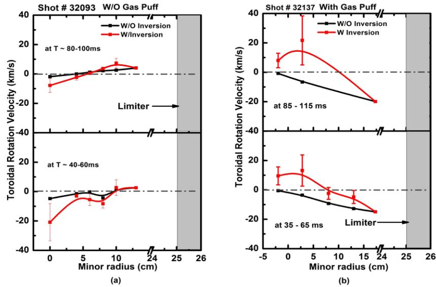
FIG. 6. Shows toroidal rotation velocity profile along with error bars are shown for (a) shot # 32093 without gas puff and (b) shot # 32137 with gas puff
