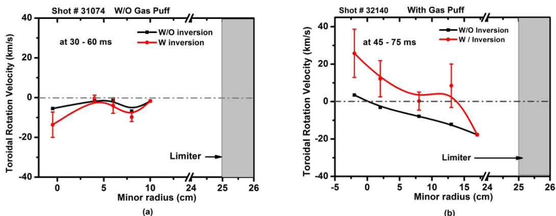
FIG. 5. Shows toroidal rotation velocity profile along with error bars are shown for shot # 31074 without gas puff and shot # 32140 with gas puff
