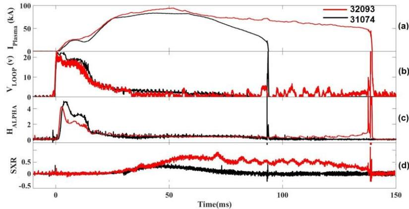
FIG. 2. Typical ADITYA-U discharge of shot #32093 along with CCD exposure duration.(a) Plasma current, (b) loop voltage (V), (c)  $H_\alpha$  emission and (d) soft X-ray emission(SXR)
