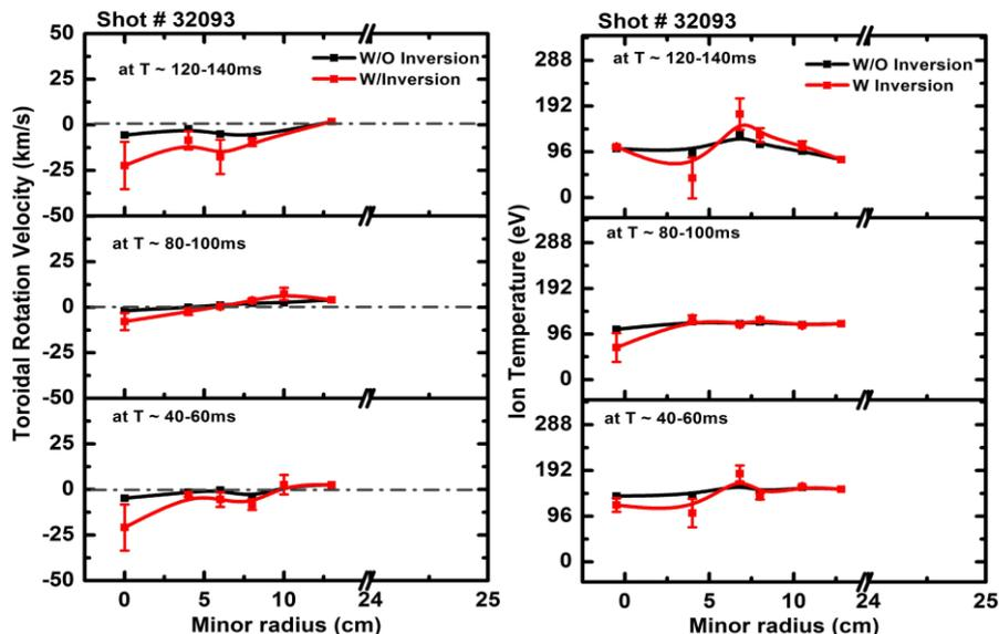
FIG. 4. Temporal evolution of toroidal rotation velocity and ion temperature profile along with error bars are shown for shot # 32093
