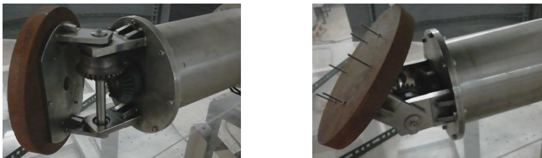
FIG. 9. ARIA Payload demonstration (A) J5 Yaw Full range test (B) J5 Pitch Full range test
