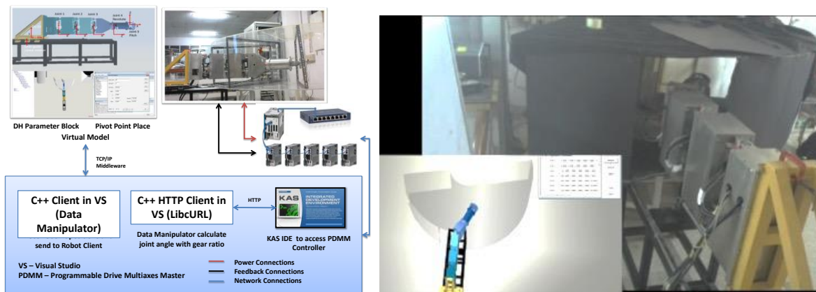
FIG. 5: Block diagram of VR based control system (A) VR based controlling of ARIA arm (B)
