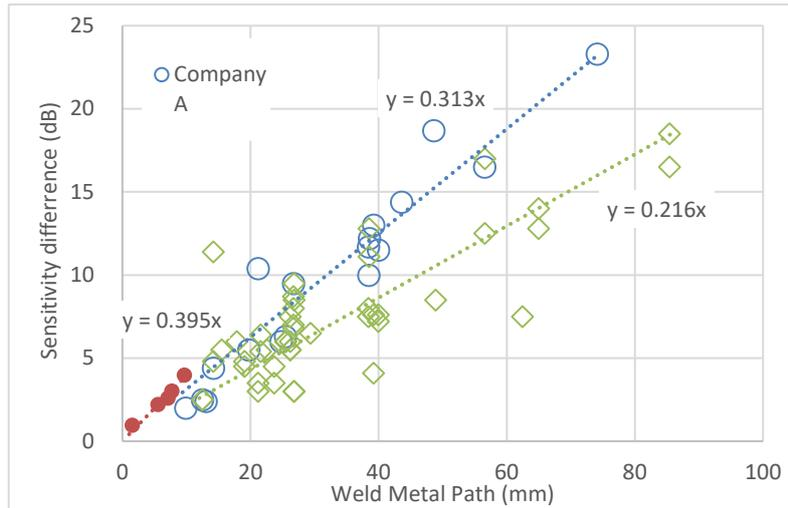
FIG. 8. Sensitivity difference by propagation distance through weld metal
