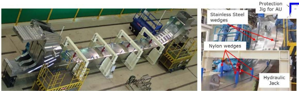
FIG. 10. AU-AP Fitting Test (Left) and guide jigs to control the position of AP (Right)
