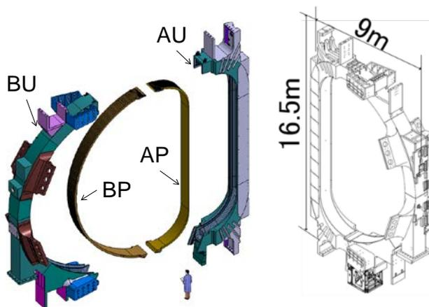
FIG. 1. ITER TF Coil Structure
