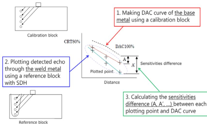
FIG. 7. Concept of sensitivity setting for attenuation by weld metal
