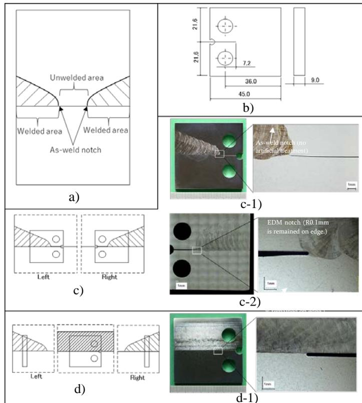
FIG.3 Information for mock-up and CT specimens, a) illustration of mock-up having actual PPW joint shape, b) dimension of CT specimen, c) sampling position of CT specimens for as-weld and EDM notch(EDM dia.0.2mm applied to as-weld notch and finally R0.1mm is remained on edge) , c-1) photograph of CT specimen having as-weld notch, c-2) photograph of CT specimen replaced as-weld notch with EDM notch, d) sampling position of CT specimens for weld metal, d-1) photograph of CT specimen for weld metal
