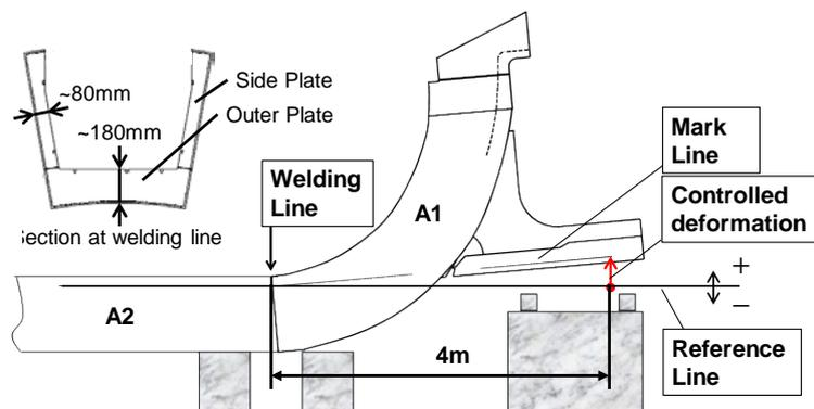
FIG. 5. Segment-to-segment welding (A1-A2)
