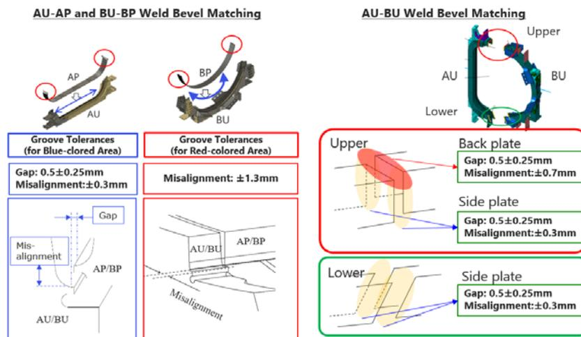
FIG. 9. Weld root matching tolerances of TFCS
