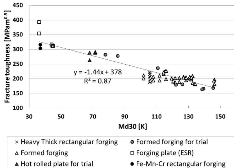
FIG.2 Correlation between the fracture toughness and Md<sub>30</sub>
