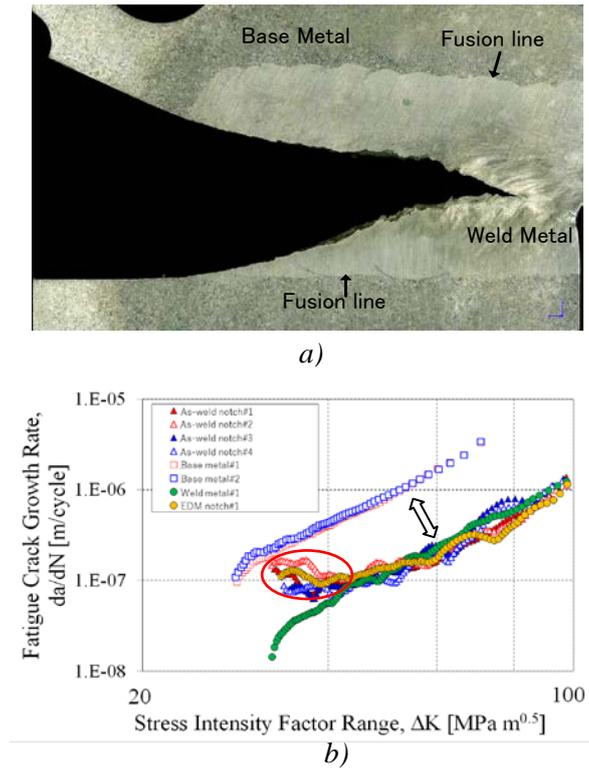
FIG.4 FCGR test result, a) Photograph overview of as-weld notch type after FCG test with etching by aqua regia, b) FCGR test results for all specimens
