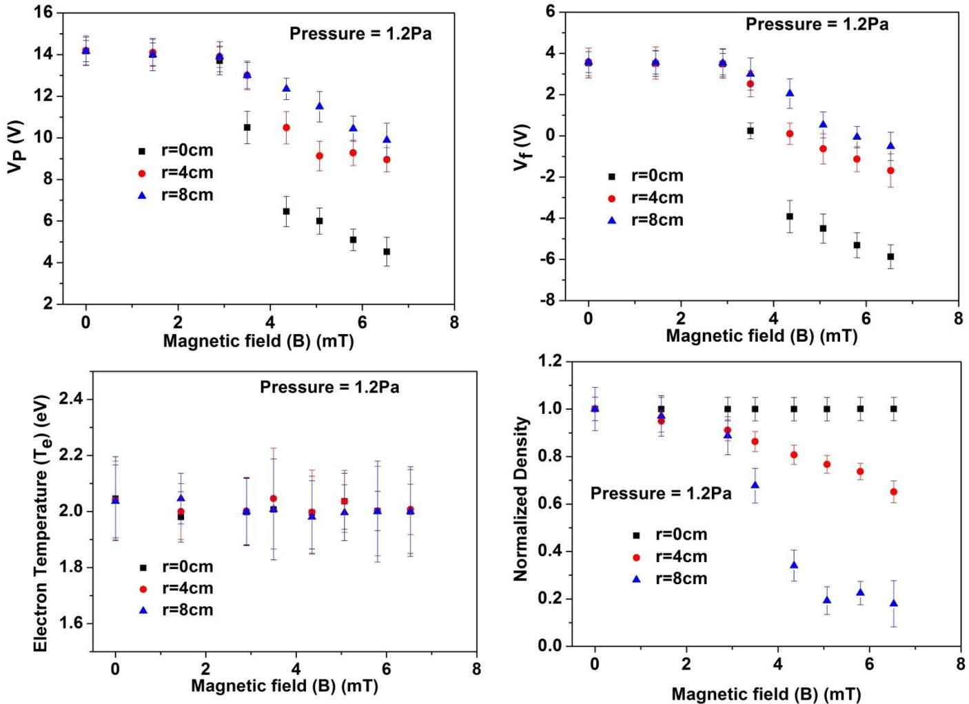
Fig.3 Different Plasma Parameters with magnetic field variation for different radial position
