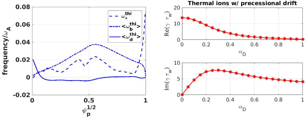
FIG. 6. Left: Frequencies for thermal ions averaged over velocity space and flux surface: precessional drift frequency (solid), bounce frequency (dot-dashed) and diamagnetic frequency (dashed). Right: scan of the drift kinetic contribution.
