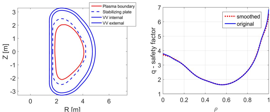
FIG. 2. Left: Plasma boundary, first wall (stabilizing plate) and vacuum vessel contours. Right: Safety factor profile before (blue) and after (red dashed) smoothing of plasma boundary and internal profiles
