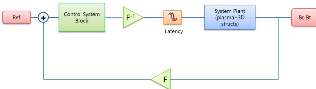
FIG 7. Block diagram of feedback system implemented in the closed loop model of RWM control
