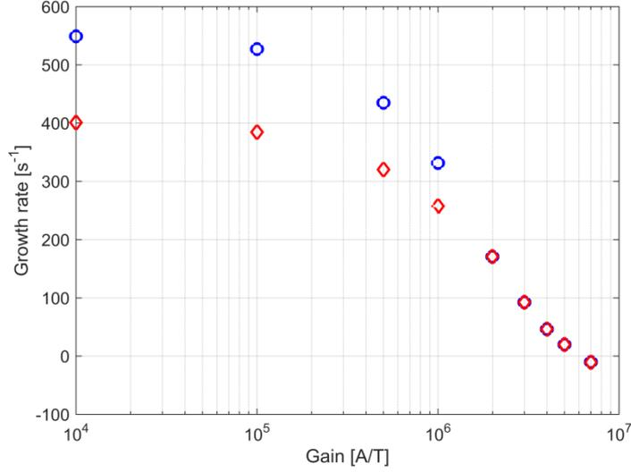
FIG. 8. Eigenvalue study of the full system with proportional controller. Two unstable  $n=1$  modes are found and stabilized at the same time.
