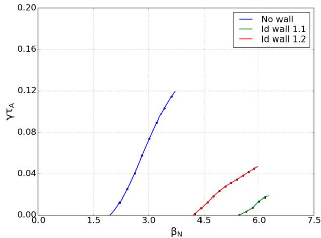
FIG. 3. No-wall and Ideal-wall stability limits calculated for  $n=1$  with constant plasma current. Two ideal wall positions are shown:  $b/a=1.205$  (red) and  $b/a=1.119$  (green)
