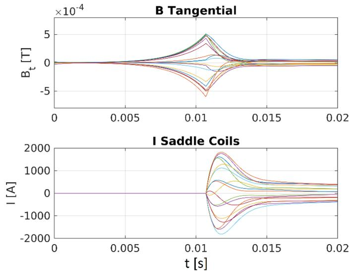
FIG. 9. Tangential field (upper plot) and coil current (lower plot) for each sensor and each active coil, example taken from the highest gain case  $K_p=8 \times 10^6$ .
