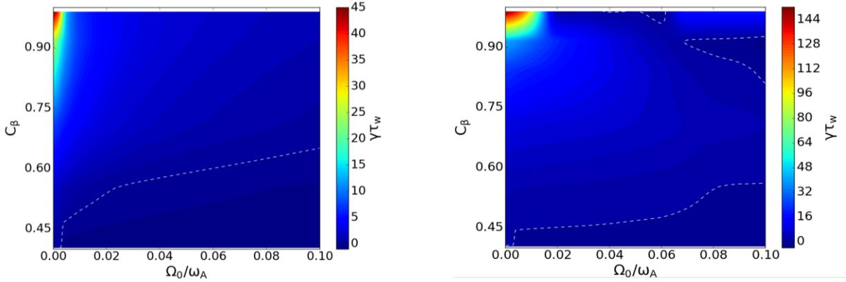
FIG. 5. Contour plots of the real part of the normalized RWM eigenvalue with varying rotation speed and plasma pressure. The fluid model is used with a small viscous damping coefficient  $\kappa_{\parallel} = 1.5$  (left)  $\kappa_{\parallel} = 0.1$  (right). Both plots use rotation profile in FIG. 4.
