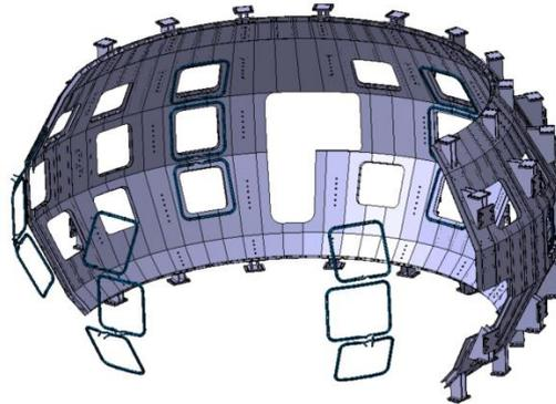
FIG. 1. 3D representation of the JT-60SA stabilizing plate and RWM control coils
