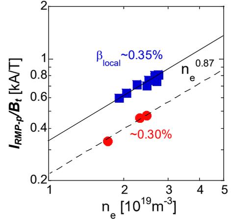
FIG. 2. RMP penetration threshold as the function of the density at the rational surface in the LHD with  $A_p=5.7$  for the  $m/n=1/1$  mode. Here  $\beta_{\text{local}} \sim 0.35\%$  ( $\blacksquare$ ) and  $\sim 0.30\%$  ( $\bullet$ ) are shown.
