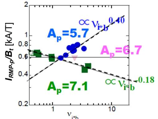
FIG. 3. RMP penetration threshold dependence on collisionality for various  $A_p$  configurations in the LHD.  $\nu_{i^*b}=1$  means the boundary of the plateau and the banana regimes.  $A_p=5.7$ , 6.7 and 7.1 are shown by  $\bullet$ ,  $\blacktriangledown$  and  $\blacksquare$ , respectively.
