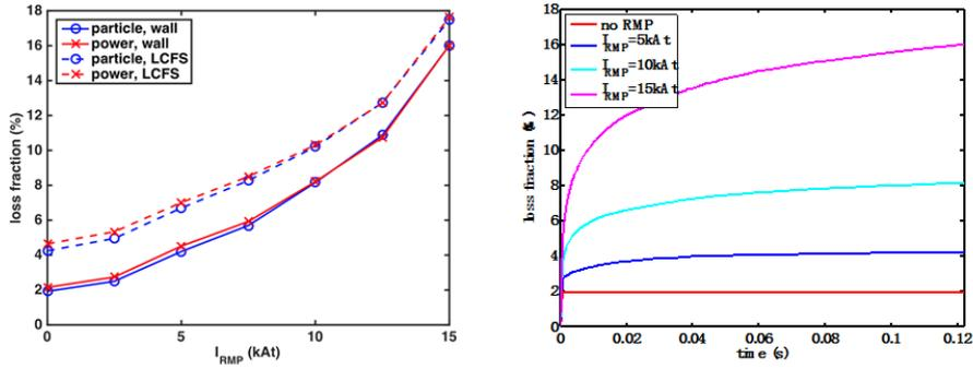
FIG. 9. Loss fraction of fast ions as a function of the RMP coil current and time, respectively.
