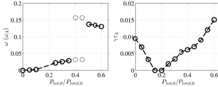
FIG. 1. Mode frequency and linear growth rate as a function of fast ion pressure fraction.
