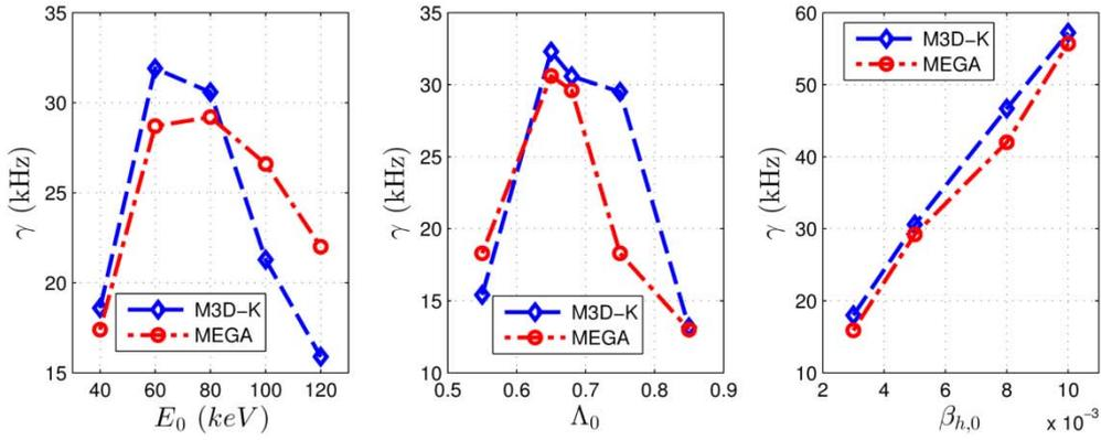
FIG. 7. The TAE growth rate as a function of beam injection energy, pitch angle parameter, and beam ion central beta.
