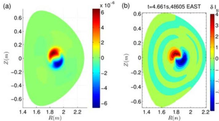
FIG. 2. Mode structure of fishbone instability. (a) M3D-K simulation result; (b) EAST experimental measurement.
