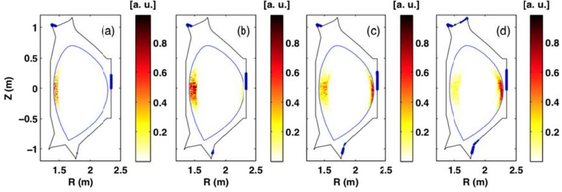
FIG. 10. Initial and final positions of lost fast ions. (a) without RMPs; (b)  $I_{RMP}=5$  kAt; (c)  $I_{RMP}=10$  kAt; (d)  $I_{RMP}=15$  kAt.
