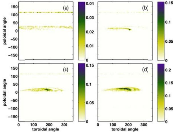
FIG. 11. Heat load for different RMP coil currents. (a) without RMPs; (b)  $I_{RMP}=5$  kAt; (c)  $I_{RMP}=10$  kAt; (d)  $I_{RMP}=15$  kAt.
