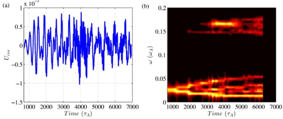
FIG. 3. Time evolution of the mode amplitude and frequency of the fishbone instability.
