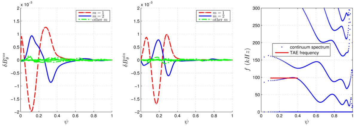
FIG. 5. Radial profiles of poloidal harmonics of the perturbed poloidal magnetic field, and the Alfvén continua with  $n=-1$ .
