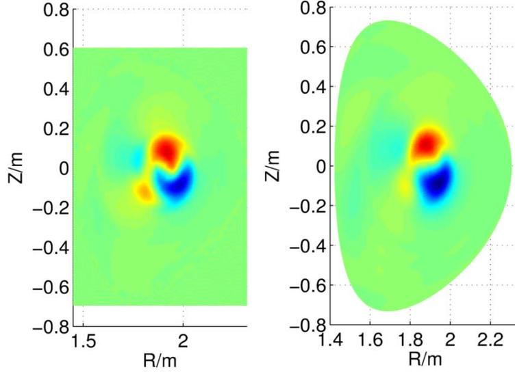
FIG. 6. Mode structure of the TAE. Left: MEGA simulation result; Right: M3D-K simulation result.
