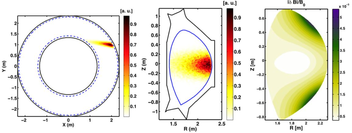
FIG. 8. NBI deposition (left:top view;middle:poloidal cross-section) and RMPs (right) on EAST.
