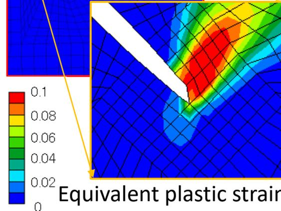
➔ The crack propagation is not likely to occur.
