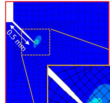
The crack tip blunting does not occur due to hardening.
