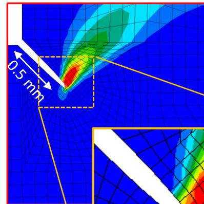
➔ The crack propagation is not likely to occur.
