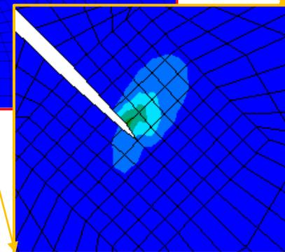
The crack tip blunting does not occur due to hardening.
