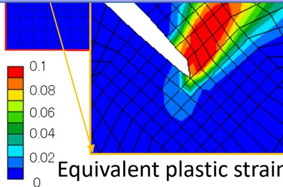
The crack tip blunting does not occur due to hardening.
