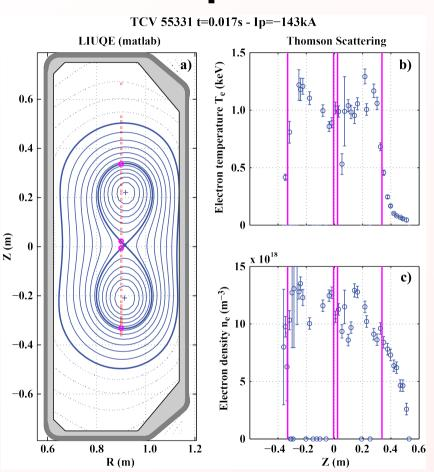
ECH-assisted Doublet showing **two hot lobes** and a cool mantle (see RHS with Thomson Ne and Te profiles with vertical lines showing reconstructed lobe positions)
