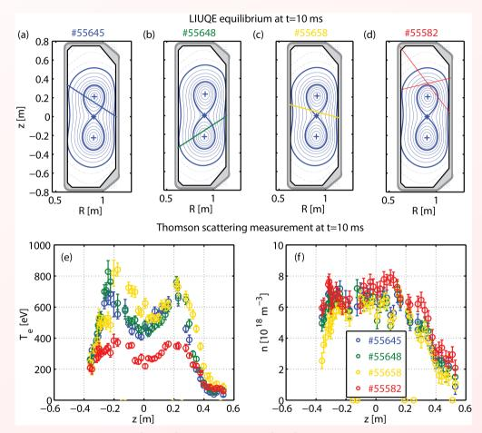
Thomson Profiles for a range of **ECH heating locations**. With heating in one or the other lobe, the profiles are remarkably similar. With a cold mantle, this could be **explained by a barrier** just outside the LCFS
