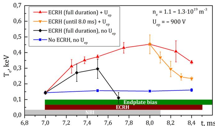
One gyrotron was used to produce pre-plasma by microwave discharge, another one heated the plasma. Central parts of segmented endplates were electrically biased to suppress MHD activity at the near-axis region. Electron axial losses:  $\langle E_e \rangle = 4.6 \pm 0.4 T_e$ .
