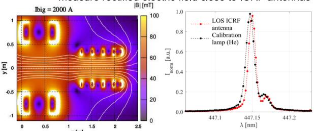
Electric field can be measured using the Stark Effect
