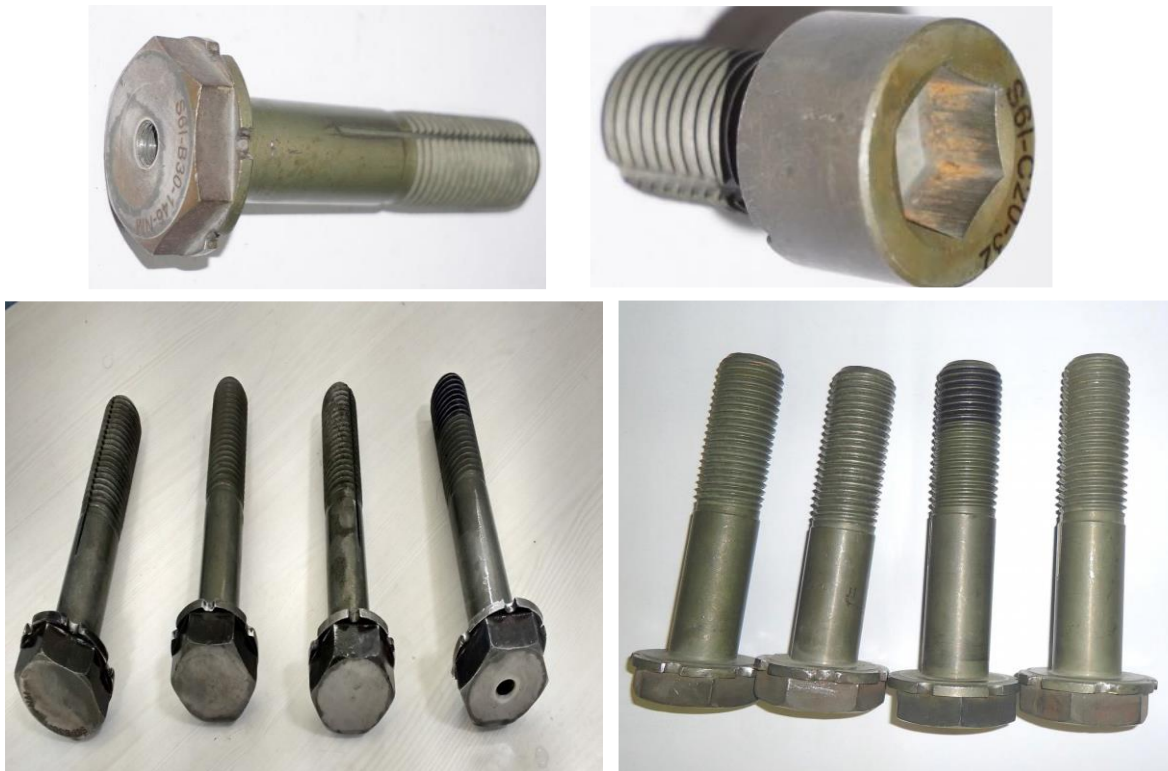
Fig.2 IWS fasteners in oxidised condition
