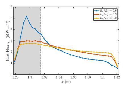
Heat-flux to divertor plate profile. Width narrows at highest poloidal field.
