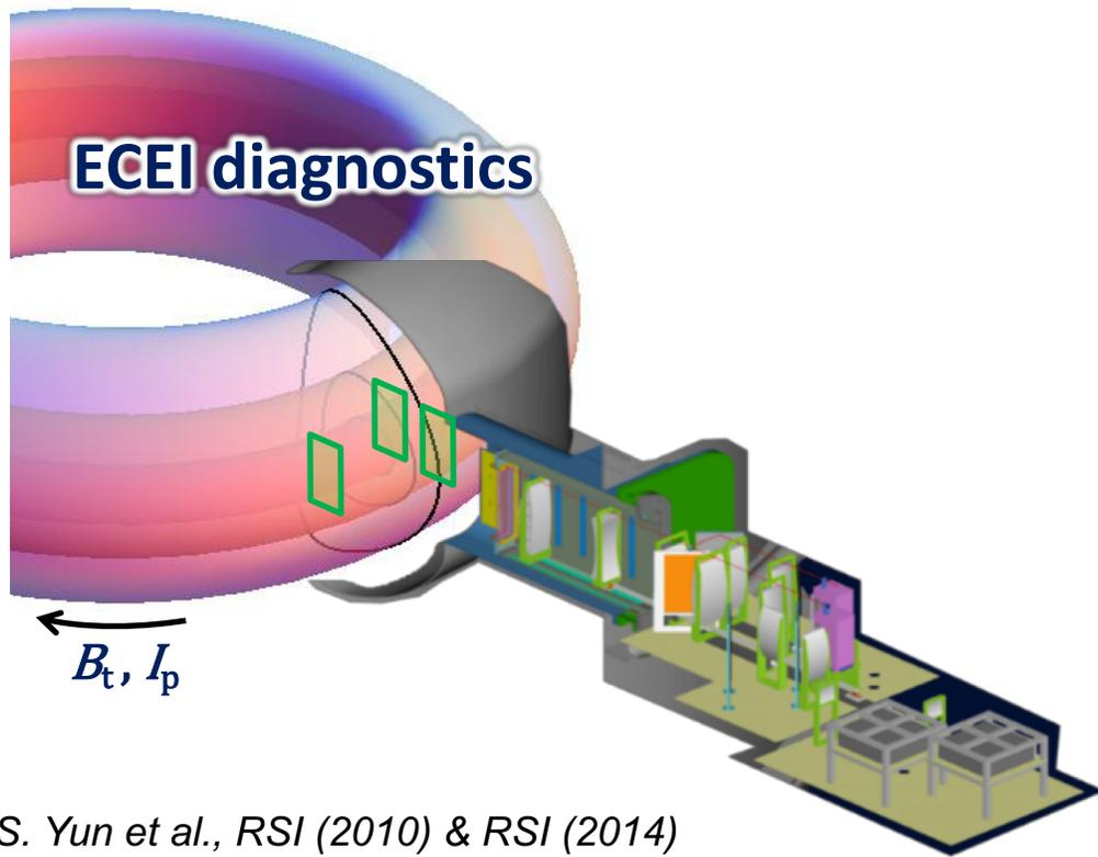
Each ECEI system is composed of 24x8 channels
