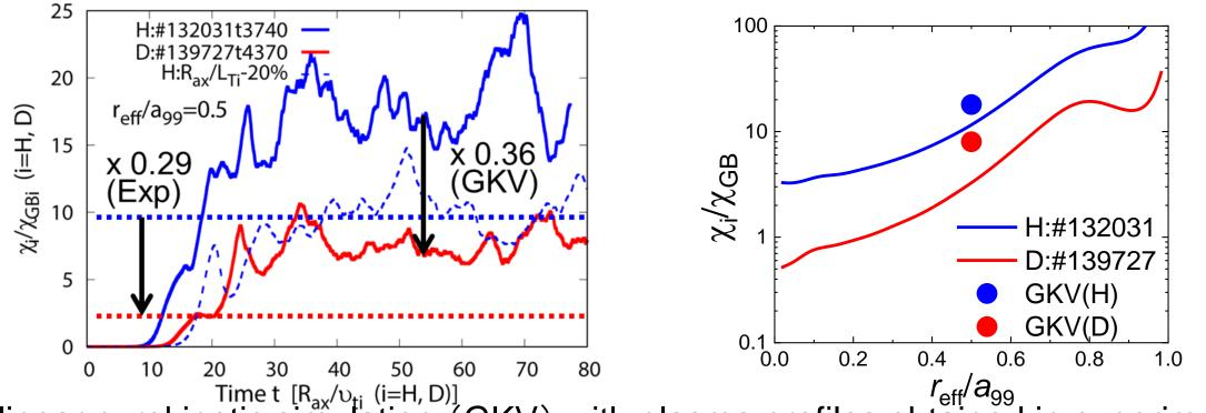
Time t  $[R_{ax}/v_{ti} (i=H, D)]$ Nonlinear gyrokinetic simulation (GKV) with plasma profiles obtained in experiment
