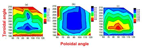
Performance of 230GHz ECCD (Za = 0 m) (a) ECCD (kA/MW); (b) Peak location of  $J_{CD}$ ; (c)  $2^{nd}$  Harmonic absorp. ratio (%)
