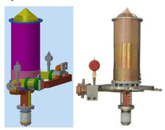
4.6GHz 500kW/CW Klystron model and structure
