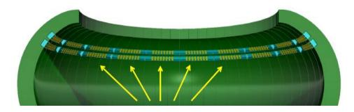
Traveling wave antenna modules arranged in the blankets, satisfying high power requirements
