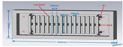
Helicon waves traveling wave antenna module
