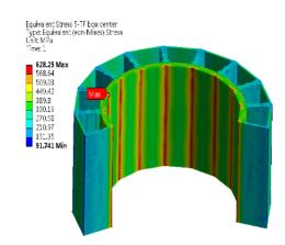
Max Force @TF coil ~736 Mpa; Max. Deformation ~ 16.5 mm
