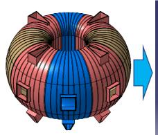
H  $\sim$ 15 m , W  $\sim$  9.1 m , Thickness  $\sim$ 50 mm , 8 Sectors, 4/6/8 ports
