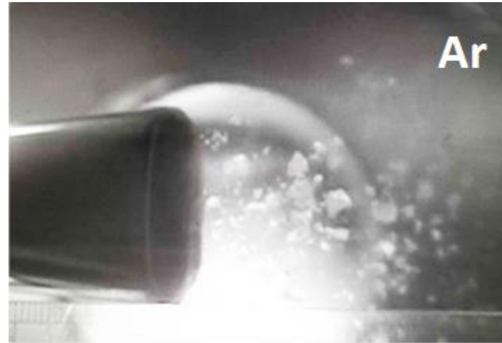
Shattered argon 12.5 mm pellet
