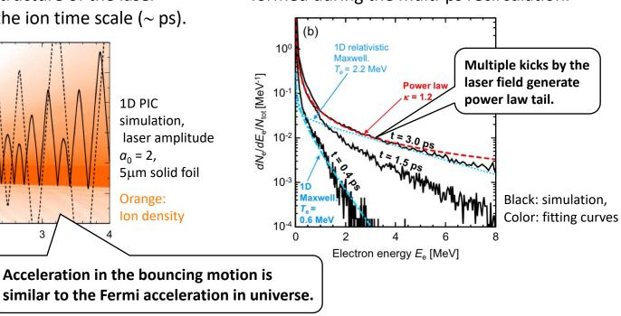
Superthermal electron generation by ps lasers discussed here can be a basis for laboratory applications and also can provide a key to understand astrophysical phenomena such as cosmic ray acceleration.
