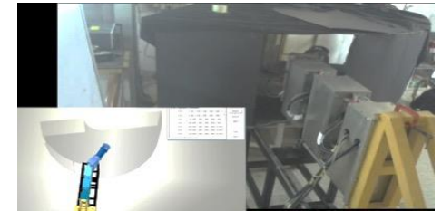
VR based controlling of ARIA arm
