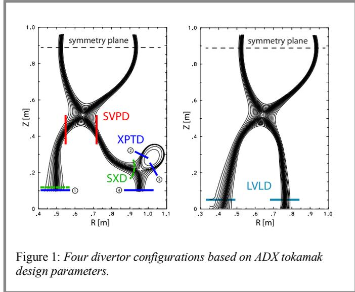
Figure 1: Four divertor configurations based on ADX tokamak design parameters.
