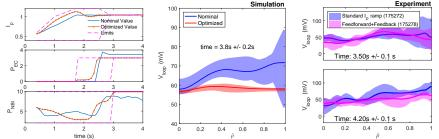
Feedforward control is combined with model-predictive feedback control (real-time optimization) to help track a plasma state evolution that is predicted to evolve to a flat loop voltage profile
