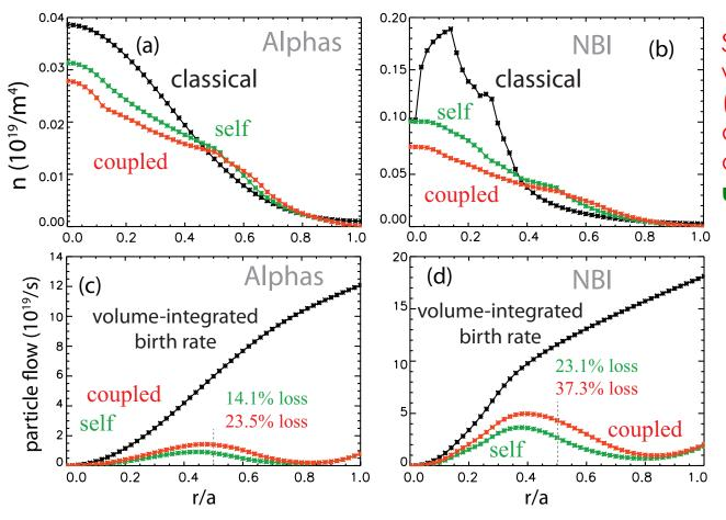
Self-consistent transport with **coupled drive** (simultaneous drive by alphas and NBI ions) is about **50% larger** than **uncoupled transport**.
