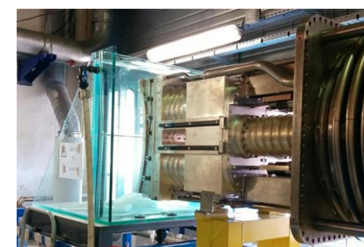
Set-up: aquarium with salted water Distance aquarium \leftrightarrow straps is adjustable
