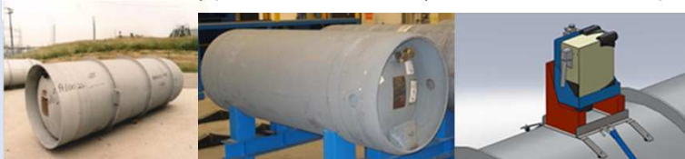
30B container (D 76cm) 48Y container (D 122cm) Measurement config.
