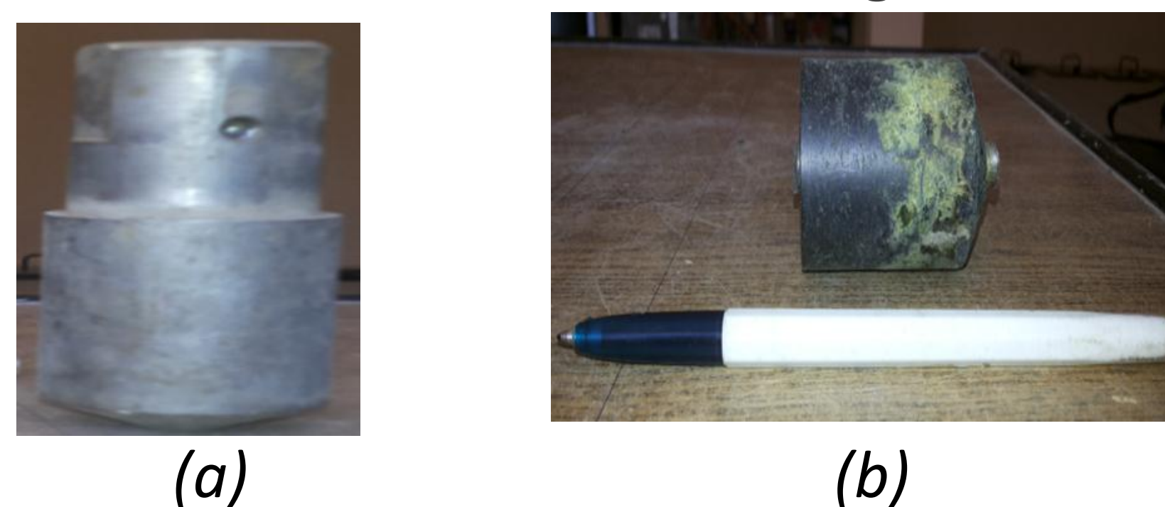
Fig. 1: The outer shape of DU container sample (#1) (a) with and (b) without its cladding.
