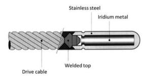
FIG. 1. Iridium-192 source for HDR BT (courtesy of Nucletron, Netherlands).
