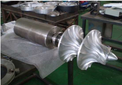
Fabrication of Impeller
