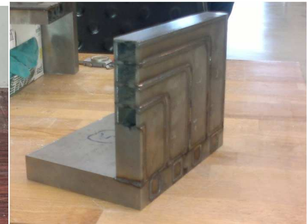
L-Shaped He Channels in the Back Plate
