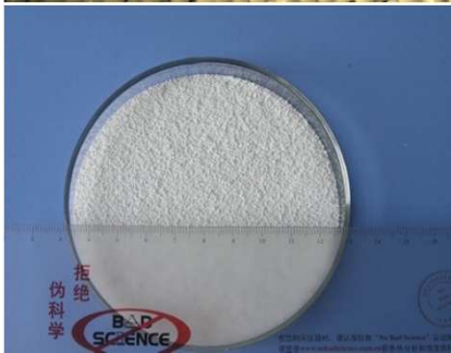
\text{Li}_2\text{TiO}_3 Pebbles (D=1mm) by Sol-gel method@CAEP
