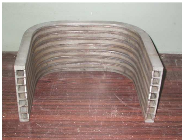
First Wall Mock-up fabrication by Laser Welding
