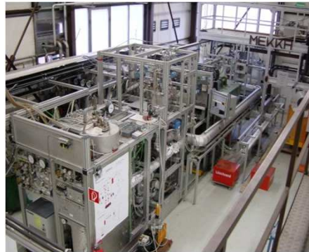
The MEKKA facility at FZK NaK loop for MHD experiments
