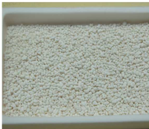
After sintering at 1000^\circ\text{C} , 6 hours, by Solution Combustion Process
