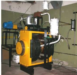
PbLi loop at IPUL for corrosion experiments.
