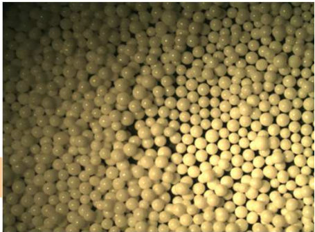
Main properties ( \text{Li}_4\text{SiO}_4 ) by melt spraying method
