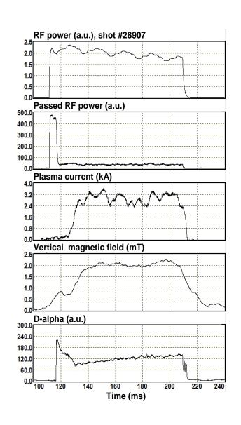
Special experiment was done with the constant poloidal magnetic field when the poloidal flux created by vertical field remains constant.
