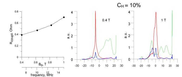
Antenna-plasma coupling resistance raise increases RF power absorption efficiency with magnetic field
