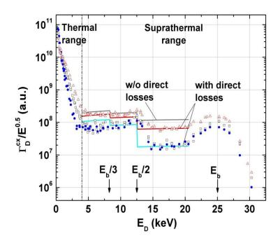
NB heating may be more efficient in Globus-M, but big losses of fast particles from bad orbits are recorded.
