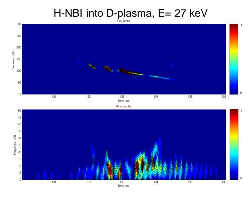
MHD fast particle instabilities do not introduce additional fast particle losses. High frequency (upper box) MHD and low frequency instabilities driven by fast particles are recorded.
