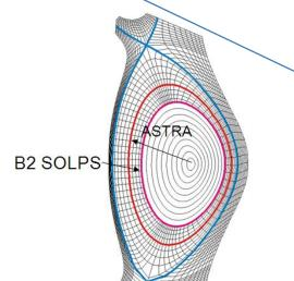
Simulation results of 1-D ASTRA transport code and 2-D B2SOLPS. Both codes were used in a serial-iterative manner to simulate the plasma periphery and the SOL in Globus-M.
