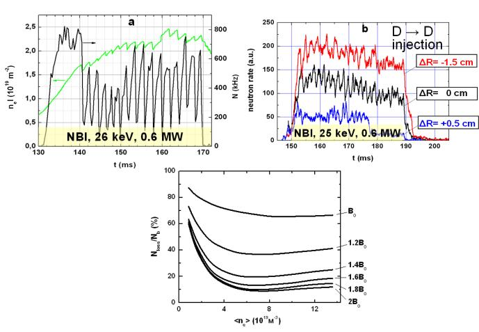
Additional losses are connected with sawteeth development. The coincidence of sawteeth phase and fast particle flux of high energy is recorded. After sawteeth start the flux of fast particles drops sharply.
