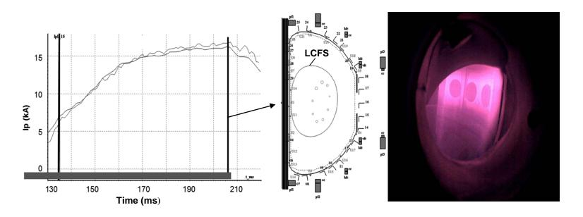
When the plasma current is les than 50 kA it is difficult to reconstruct by standard EFIT code.
