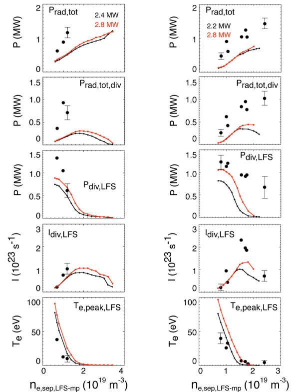
**EDGE2D/EIRENE predictions of power, currents and electron temperature for an identical grid and boundary conditions in JET-C and JET-ILW**
