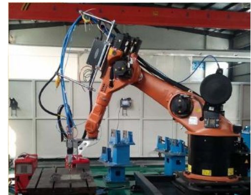
Welding robot with a 4kW fiber laser welding equipment
