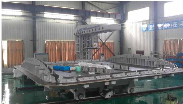
CC winding table with Side Correction Coils mold
