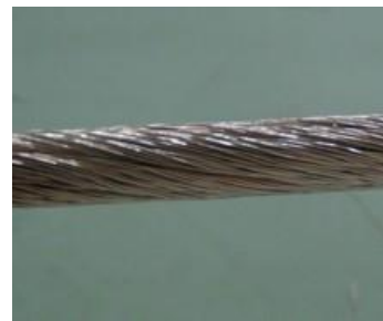
CC sc Cable at ASIPP
