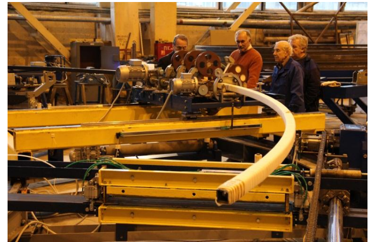
Conductor turn insulation trial
