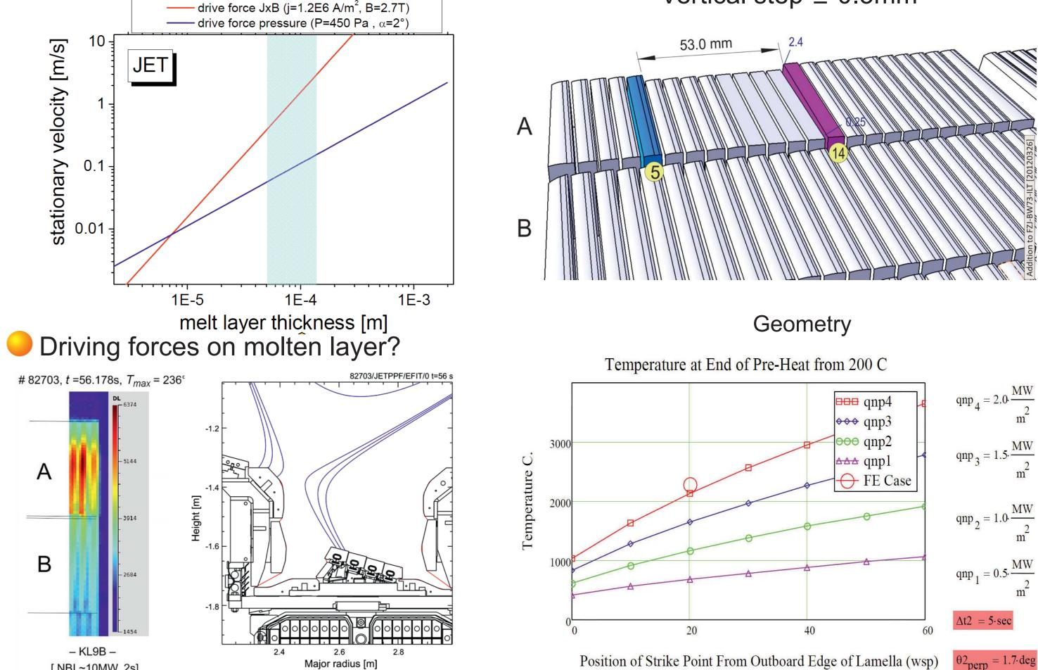
Unique: Melting in 2 steps, steady state pre-heating + large ELMs Operation on 'stack A' Evolution of melt damage and power handling? The dedicated experiment planned in JET may provide *in fine* a significant contribution to the decision on a full W divertor [3] from the very beginning in ITER.
