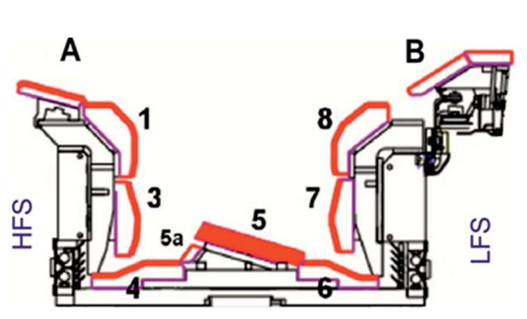
The new divertor coating configuration is as follows: Tiles A, 3, 4, 5a  $-12 \ \mu m$  Mo/W. Tiles 1, 6, 7 and 8  $-25 \ \mu m$ Mo/W or Mo/W/Mo/W. Mo layers are  $\sim 2\mu m$  thick in all cases
