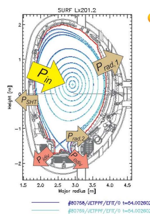
Power balance with corrections in the order of 10%: deposited energies in the outer divertor ~ 20-30  $MJ/m^2$
