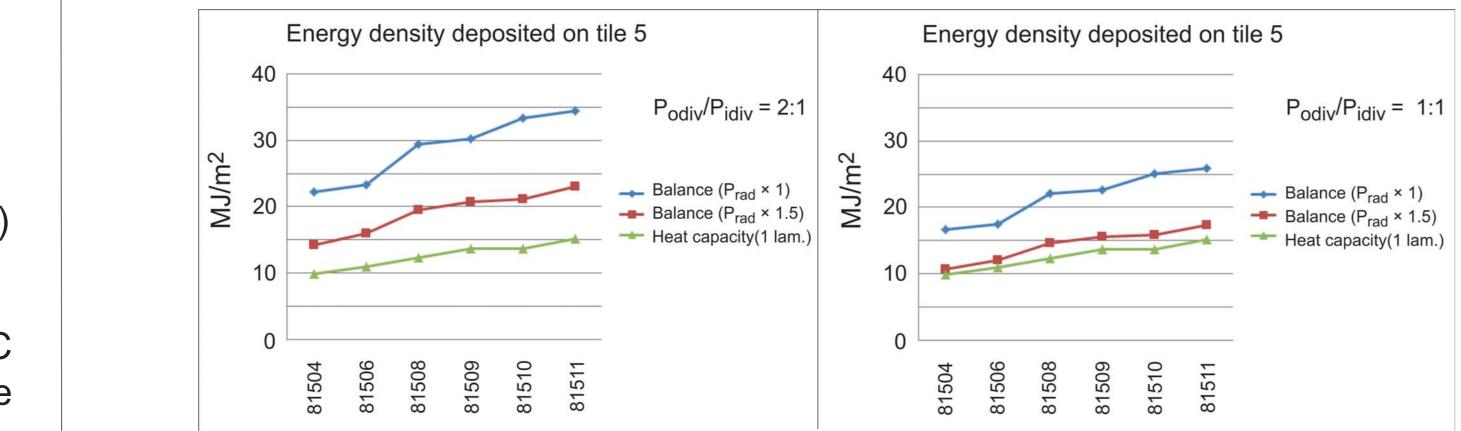
NB pulses with both ISP and OSP on the vertical targets tend to confirm a 2:1 power sharing between the legs -
