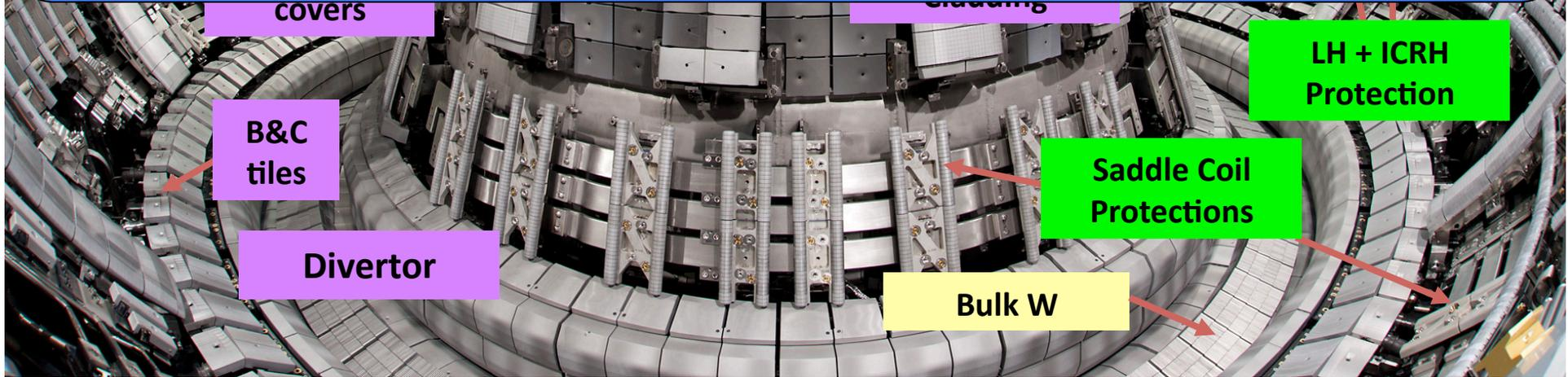
**ILW = 2880 installable items, 15828 tiles (~2 tonnes Be, ~2 tonnes W)**
