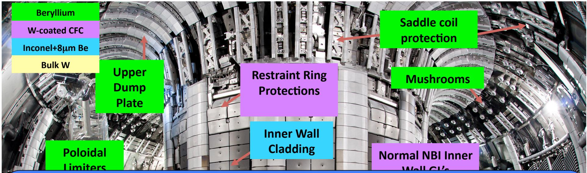
JET is now equipped with the same combination of materials as ITER, up to 34MW of NB power and improved diagnostic and control tools.
